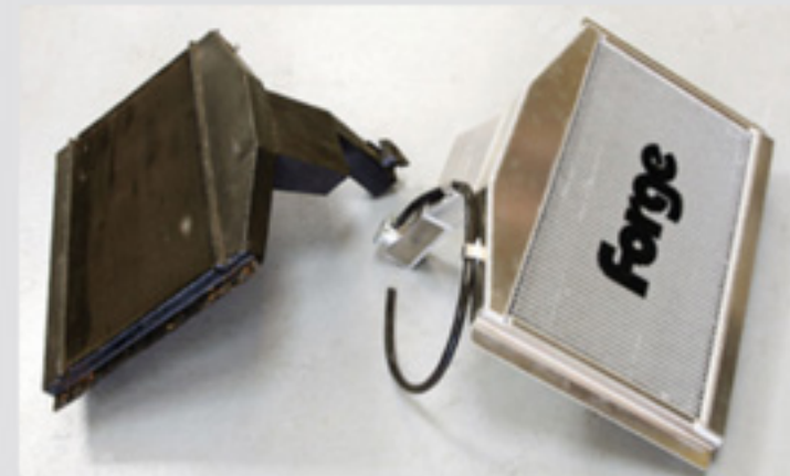
Super-efficient radiator core and use of aluminium will improve cooling way beyond the limits of the original.
