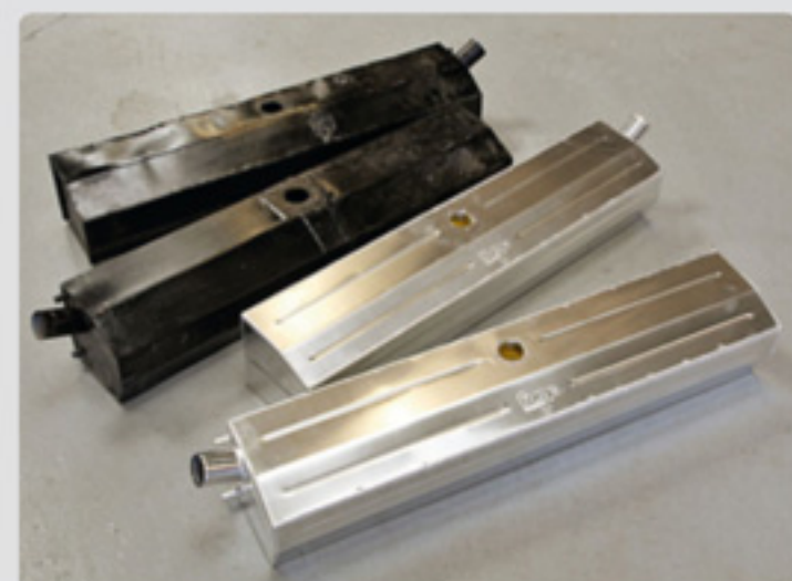
Lighter stronger, safer. The twin fuel tanks are a world away from the marginal, tired originals.
