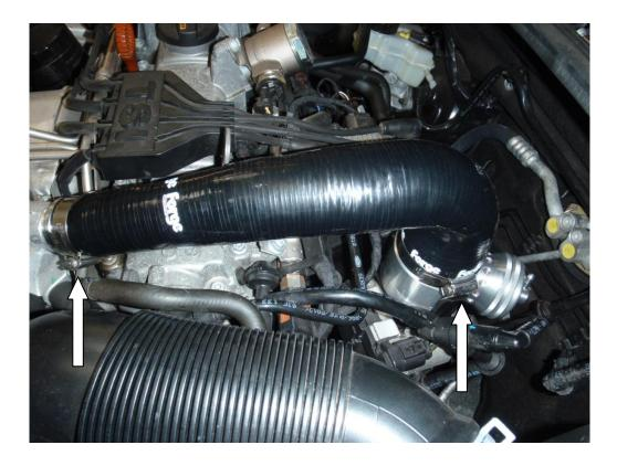
8. Unclip the second map sensor from the inlet manifold and insert the alloy take off.9. Insert the map sensor into the alloy take off and secure using the provided self tapping screws.
