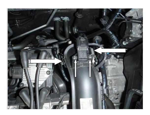
4. Remove the rubber O ring from the plastic boost pipe and insert into the alloy dump valve adaptor
