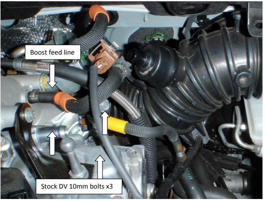
8. Fit the supplied Forge blanking plate to the turbo, reusing the bolts you removed in step 8.
