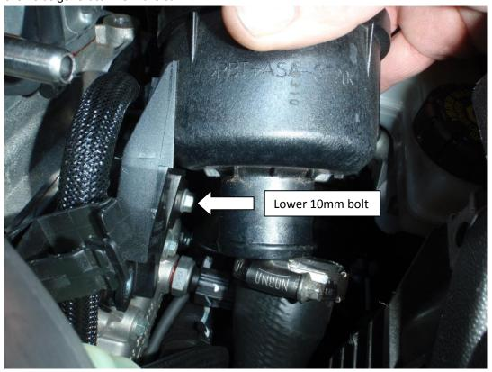
6. Locate the vacuum feed to the standard valve as shown below. Remove the rubber feed to the valve from the stock tee piece.
