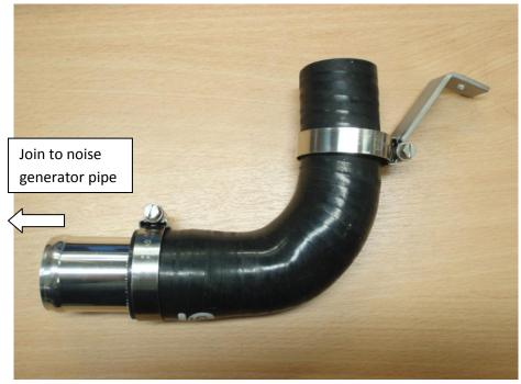
10. Fit the valve to the end of the pipe and tighten the jubilee clip whilst positioning the bracket over the hole in the firewall. Use the bolt and plain washer on the top of the bracket, and penny washer and nyloc nut on the bottom to secure the bracket. Connect the vacuum hose between the top of the valve and the tee piece in step 6 and the installation is complete!
