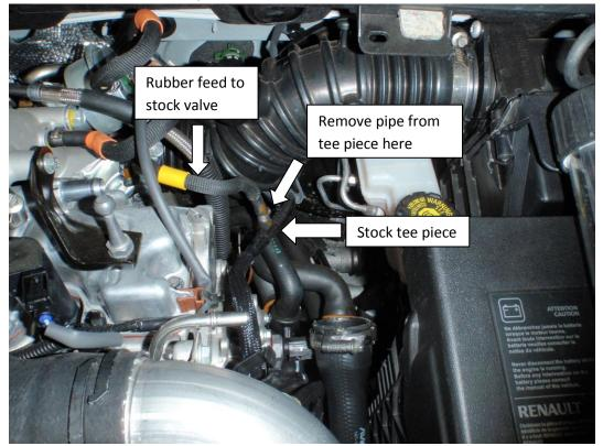
7. Remove the stock valve from the front face of the turbo by undoing the three 10mm bolts. You may find it easier for access to remove the boost feed line, and maybe the inlet pipe from the airfilter to give you more room.
