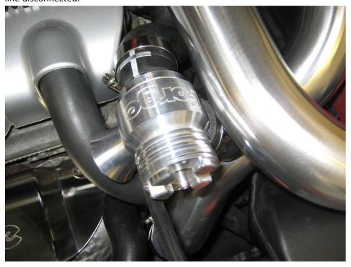
9. You now need to adjust the tension on the spring – the Split-R is fitted with a conical spring which can be adjusted to suit the boost you are running. Adjustment is made by turning the castellated top part of the valve either clockwise to INCREASE the tension or anticlockwise to DECREASE the tension. The adjuster is ratcheted so as it's turned it will 'click'.
