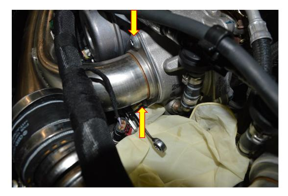
6. On the underside of the intake pipe there is a breather fitting that needs to be removed from situ, depress both the sides of the fitting while pulling the fitting away from the inlet pipe.
