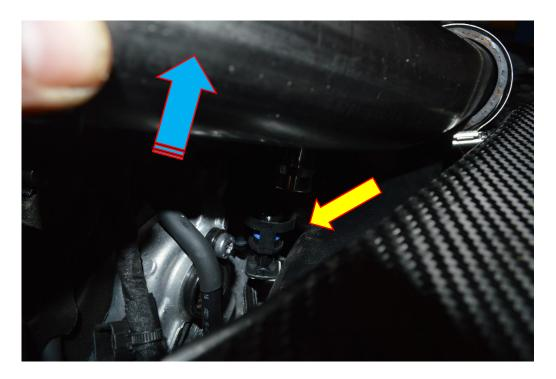
7. Using a T30 Torx drive and a small rachet remove the two fasteners that hold the right-hand side inlet pipe in situ. Follow the breather that attaches to the inlet pipe, at the end of the breather pipe the connector will need to be removed, depress the two sides as in figure 6 and the intake pipe will be released from position.
