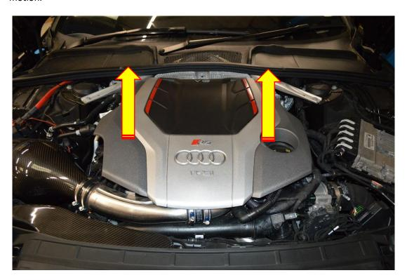
2. Using a trim tool remover or flat bladed screwdriver pry the clips that hold the wiring loom away from the inlet tracts as arrowed below.
