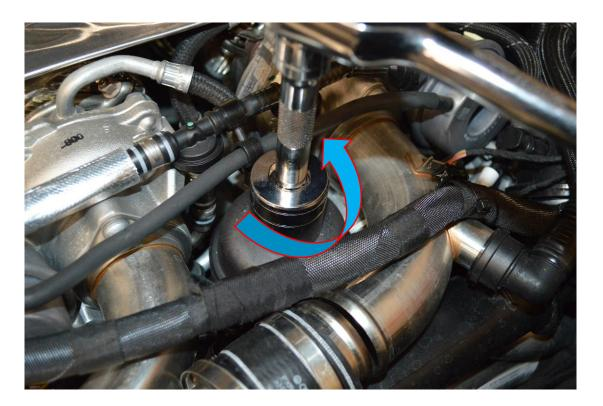
5. Using a T30 Torx drive and small rachet remove the two fasteners that attach the inlet pipe to the turbo.
