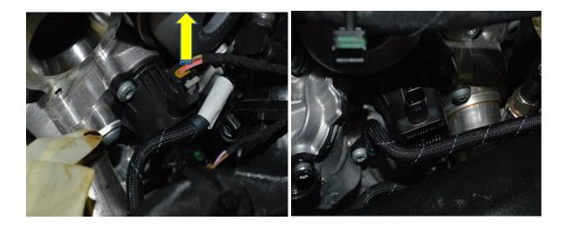
9. Using a T30 Torx remove the X3 M6 fasteners attaching each valve.
