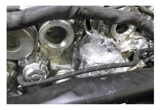
11. Starting with the left-hand side valve, connect one of the wiring looms supplied with the FMDV27 kit to the OE valve wiring loom. Run the loom under the oil breather and connect one of the solenoids from the FMDV27 kit.
