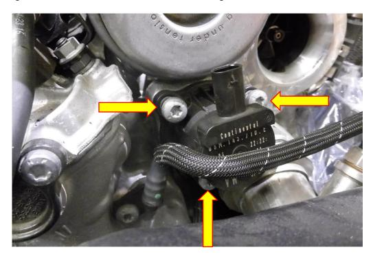
10. Ensure the supplied O-rings are in place on the base of the Forge Motorsport valves then attach the valves into the mounting position taking note that the valves are handed for the left- and right-hand turbo, this is to avoid interference with the turbo's actuators. Re-use the removed torx fasteners on each valve to secure them into position.
