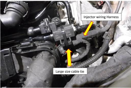
15. Run the second vacuum hose along with the actuator pipe, use the medium size cable ties provided to secure it. Mount the remaining solenoid from the kit to the injector/coil pack wiring harness and secure it with a large cable tie. Run the silicone hoses to from the valve to the solenoid as described in step 12. Attach the wiring harness from the kit to the solenoid and the vehicles DV wiring loom.
