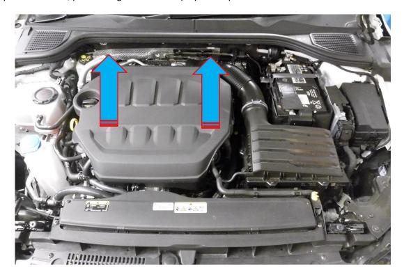
2. Using a hose clamp removal tool and a 7mm socket and ratchet, loosen off both hose clamps attaching the OE intake hose to the air box and turbo adaptor.
