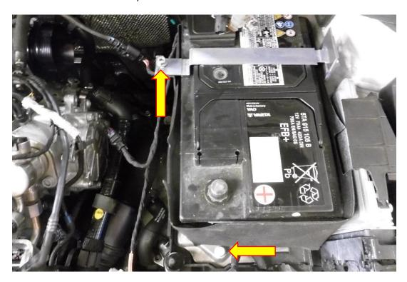
**11.** Using a 13mm socket and ratchet remove the fastener attaching the bracket to the battery tray. Remove the bracket and turn 180 degrees then re fit and fix it back into place.
