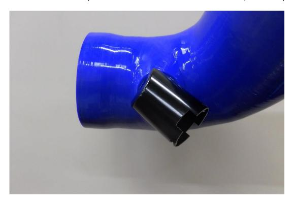
14. Take one of the supplied hose clamps and loosely place it at the turbo end of the silicone intake hose. Fit this end to the machined turbo adaptor fitted in step 6, push the breather hose into the machined breather adaptor till it clicks into position. Using a 7mm socket and ratchet secure the hose with hose clamp. (The fuel pump vac line has been removed to make the picture clearer)
