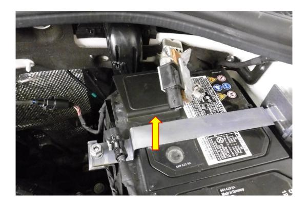
10. Using a 10 & 13mm socket and ratchet remove both fasteners attaching the clamps to the battery. You will now be able to remove the battery from the vehicle.
