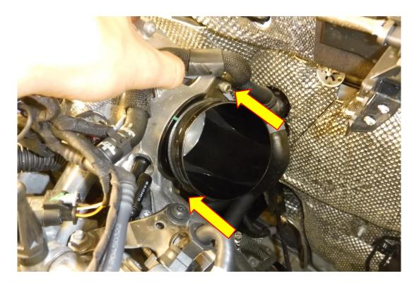
5. Using a flat blade screwdriver prise the O-ring from the OEM turbo adaptor and fit it to the Forge billet turbo adaptor.
