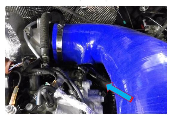
15. Using a 7mm ratchet and the remaining hose clamp attach the other end of the silicone hose to the air box.
