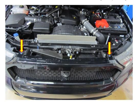
4. Locate and use a Pozi drive screwdriver to remove the two fasteners attaching the bottom of the grill. The grill will now come away from the bumper.
