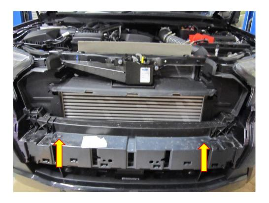
6. Using a pozi drive screwdriver to remove remove the four fasteners attaching the inner arch of the bumper to the splash guard.. This is the same for both sides.
