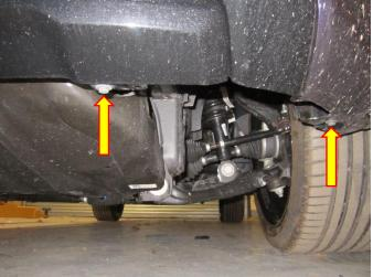
8. Remove the fastener from the inside of the splash guard attaching the bumper to the wing, do this on both sides. The bumper should now pull away from the vehicle.
