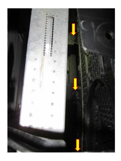
3. Using a 10mm socket and ratchet remove the two M6 fasteners attaching the top of the grill to headlights.
