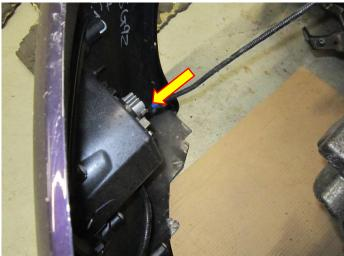
**10**. Using a 10mm socket and ratchet remove the four M6 fasteners attaching the plastic shrouds each side of the intercooler.
