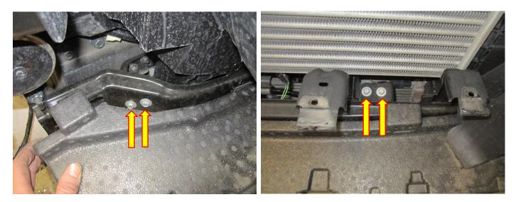
10. There are four fasteners (two each side) that attach the plastic shrouds at each side of the OE intercooler. Use a 10mm socket to remove them
