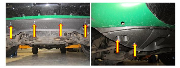
4. You will now be able to lower the valance part of the bumper downwards and access the four fasteners at that attach the bottom of the bumper to the vehicle. Remove these with a 10mm socket and ratchet.
