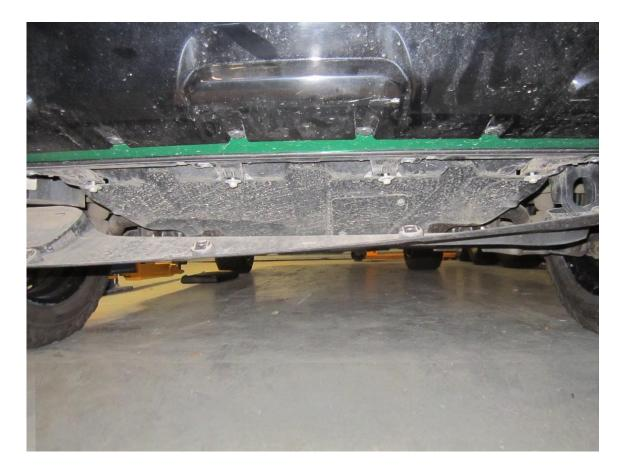
5. Use a T20 Torx to remove the fastener that attaches the inner splash guard to the bumper. With this removed you will now be able to access the fastener which attaches the top of bumper to the wing of the vehicle. Use a 10mm socket and ratchet to remove this fastener on both sides of the bumper.
