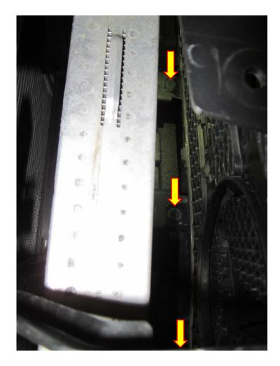
3. Use a 10mm socket and rachet to remove the eight fasteners attaching the valance to the bumper.
