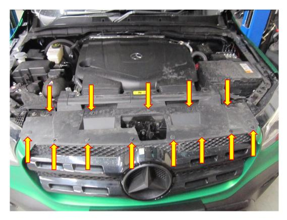
2. With slam panel cover removed you will find five plastic fasteners which need releasing. There are two at the top of the bumper and the other three are in front of the intercooler behind the grill.
