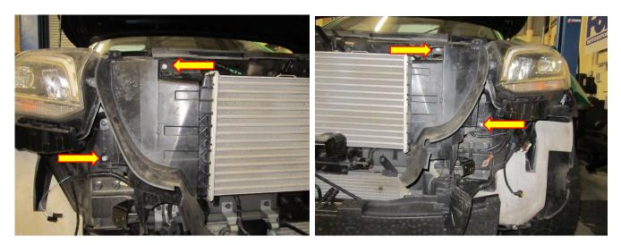
**11**. To remove the shrouds from the vehicle you need to unattach it from the air intake pipework. Use a flat blade screwdriver to push in the tabs and the shrouds will pull away from the vehicle.
