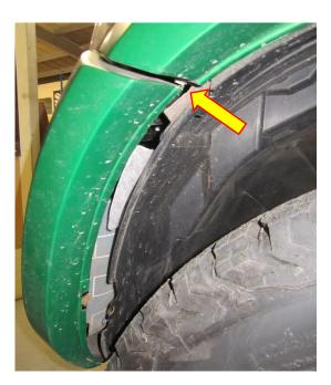
6. On the offside of the bumper you will see the hose line for the light washers, disconnect and bung up the water feed hose with a bolt or similar, to prevent water running out the system. Un-plug the fog lights on both sides also.
