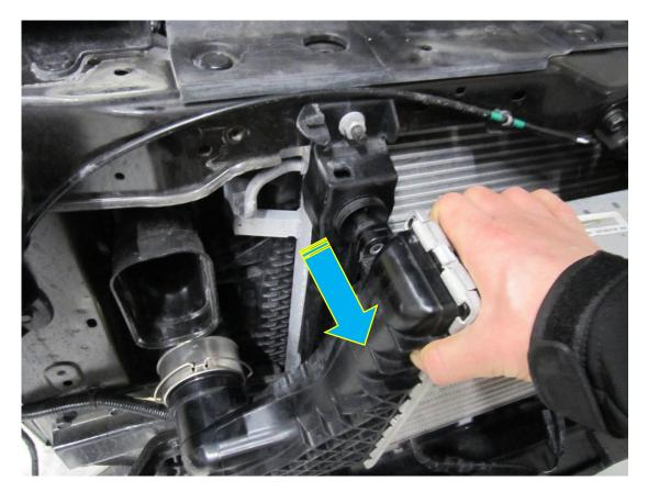
14. With the OE intercooler now removed, you will now need to remove the original mounting pegs. Use a 15mm spanner to do this, turn them anti clockwise to unscrew them.
