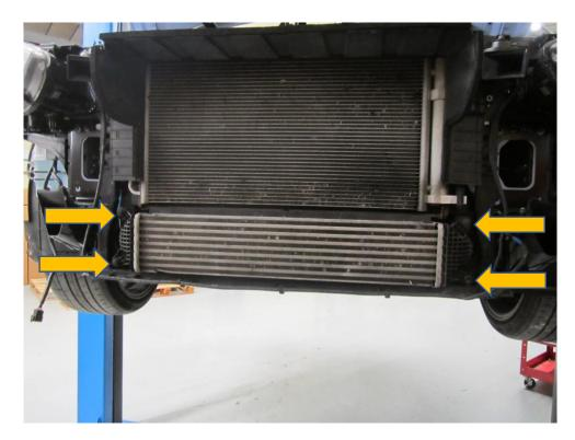
13. The rest of the off-side intercooler hose can be taken off the car, loosen the 8mm hose clamp in the same way as before, then undo the fastener holding the OE hard pipe to the car with a 10mm socket and rachet drive. Now remove the hose and pipe as one, from the vehicle.
