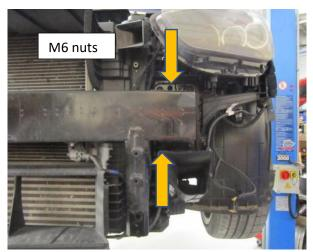
10. Removing the ducting. First unclip the wiring loom that is attached either side of the ducting by using a trim tool or flat blade screw driver to lever the retaining clip away. Using a 10mm socket and rachet drive remove the 4 fasteners holding the ducting to the car. Once they are removed the ducting can be pulled out, you may have to lever out the two locating pins at the bottom of the ducting when removing. DO NOT REFIT DUCTING WITH NEW INTERCOOLER!
