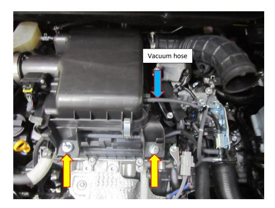
**4.** The MAF sensor will now need to be removed. First unplug the sensor, then using a Pozi-drive screwdriver, remove the two screws holding it in place. Now carefully remove the sensor from the air box. Unclip the MAF wiring harness.
