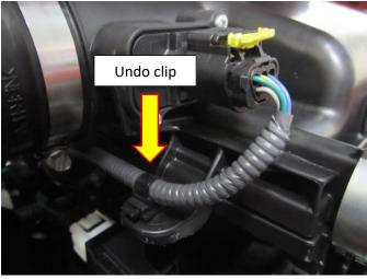
5. Remove the oil breather hose from the turbo intake pipe, this will just pull out. The hose clamp holding the turbo intake pipe also needs to be slackened off with an 8mm socket or flat blade screwdriver.
