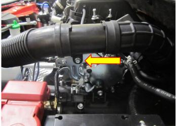
**3.** Locate the two 10mm fasteners attaching the air box to the engine, remove these with a 10mm spanner. Now remove the vacuum hose from the air box, this just pulls off.
