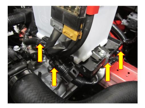
8. Slacken off the 10mm nut on the **POSITIVE** battery clamp so that you can twist it 90 degrees anti-clockwise. Pull the wiring loom around so that you can move the battery terminal into position. When you have got the terminal into the desired position, tighten the 10mm nut on the battery clamp.
