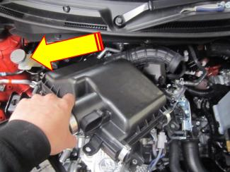
7. Before you can install the FMINDK29, you will have to relocate the positive side wiring loom to the vehicle battery. There are four plastic clips that need to be undone. Use a flat blade screwdriver to prise the clip off. At this stage, disconnect the NEGATIVE Battery terminal with a 10mm spanner/socket & rachet.
