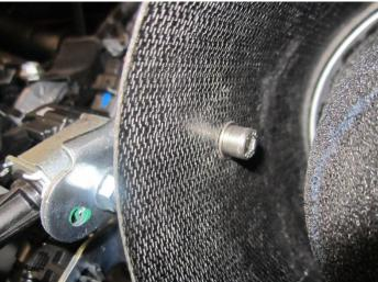
**20.** Now with the filter in place, go back to the mounting bracket and tighten the M6 fasteners and all the hose clamps for the silicone hoses.
