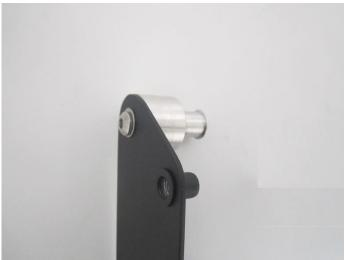
**11.** Once you have made up the mounting bracket, install it into the rubber lugs that held the back end of the airbox in place. The mounting bracket simply pushes into place.
