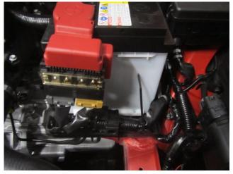
**9.** With the terminal tightened into its new position, you can now tidy the wiring loom, first tuck the excess loom around the back of the battery and cable tie it to the loom coming from the fuse box. Working backwards, cable tie the next part of the loom using the existing fastener hole.
