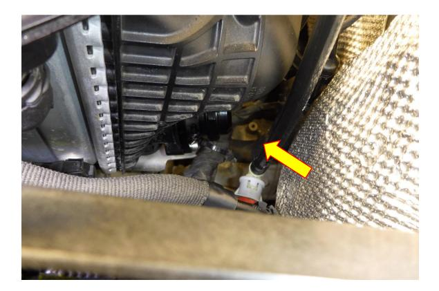
9. Use the remaining silicon hose and attach it to both ports from the Forge valve, run the hose up to the bulkhead.
