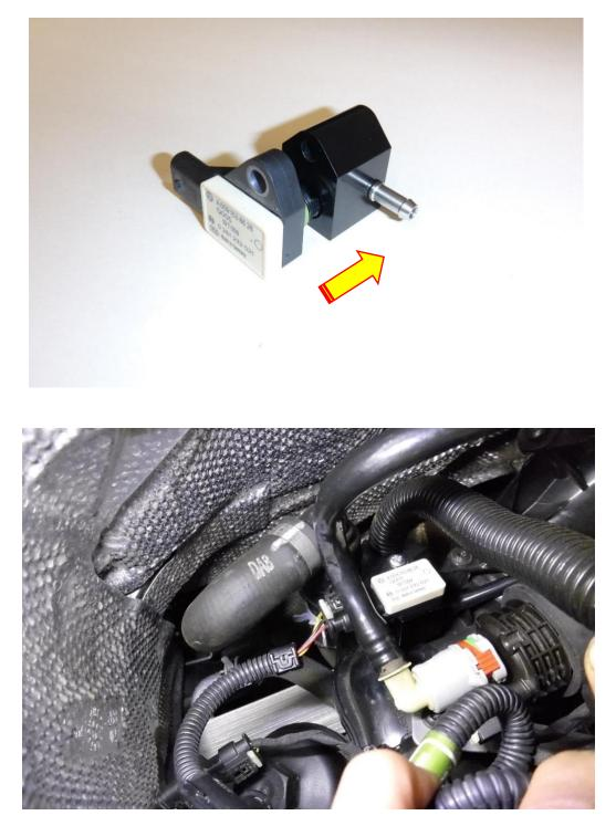
7. Run the silicon hosing along with the black vacuum pipe and use the cable ties provided to attach it.
