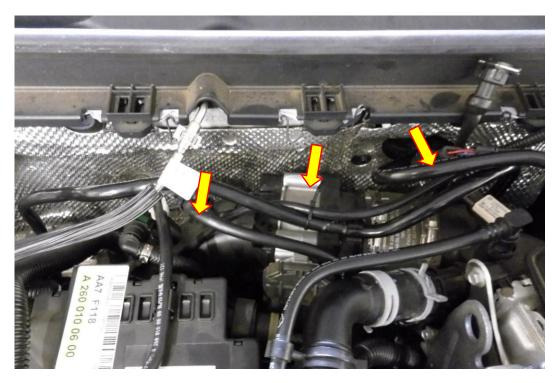
8. Fit the Forge replacement valve where the old valve was situated, secure it in place using the supplied M6x16 Allen cap head fasteners. Use a 5mm Allen key to do this. The orientation of the valve should be that the base boost port is pointing downwards.
