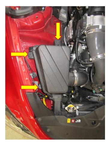
3. Next, loosen the hose clamp securing the intake pipe to the airbox, you can use either a 10mm socket and rachet or a Philips screwdriver to do this. Once loosened off the air box will lift away from the vehicle.
