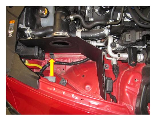
6. You will now be able to install the filter by angling the heat shield backwards and pushing the alloy filter neck through the hole in the heat shield. Insert the alloy end of the filter into the intake hose and tighten the hose clamp while pushing down on the intake hose at the same time.
