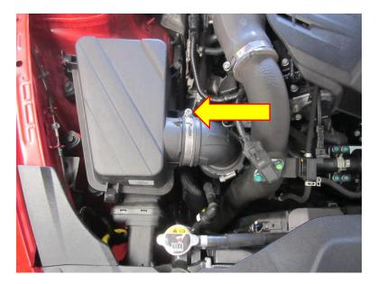
4. With both air boxes removed you can now begin to install the Forge intake kit. Starting with the offside intake, remove the nut indicated below using a 10mm socket and extension. You can now place the Forge heat shield in the engine bay, locate the middle mounting bracket on the exposed thread and secure loosely with the 10mm nut removed earlier. Do not re fit the fastener at the rear of the heat shield just yet.
