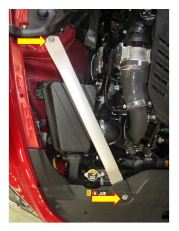
2. The air box has 3x fasteners securing it in place, remove these fasteners with a 10mm socket and rachet with an extension. This procedure is the same on both air boxes.
