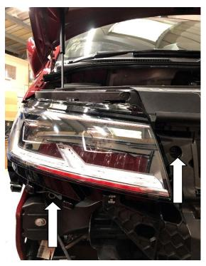
12. Unclip the wiring loom that runs along the bottom of the plastic support panel. Now remove the four T30 fasteners securing the plastic support panel, the panel will now pull away from the vehicle.
