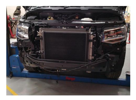
30. With the FMCCRAD10 now fitted you will have to modify the plastic support panel for it to fit back into place. Cut away all the areas marked below with a hacksaw and file.
