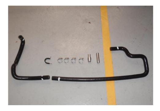
24. Fit the coolant coupler to the hose (marked #1888) provided as shown in the photo below and secure the coupler with a suitable hose clamp provided.
