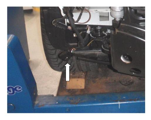
11. Loosen the fasteners for the head lights but do not remove the lights, three are T30 Torx and one is a T25 Torx.
