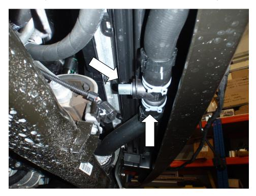
15. Using a flat blade screwdriver release the clips on the charge cooler radiator couplers.
