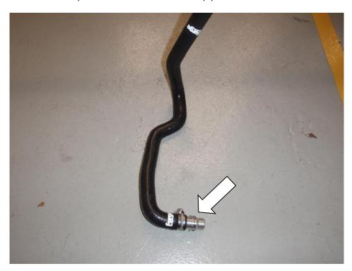
25. Connect the other hose to the outlet of the chargecooler and secure with a suitable hose clamp provided. Using the P-clip, M8 x 30mm Allen cap head bolt and the 3x 8mm penny washers provided, secure the silicone hose in position.
