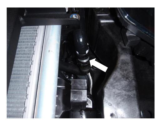
23. Using the remaining 2x hoses, 1x hose joiner, 1x coolant coupler and hose clamps, connect the second outlet of the chargecooler radiator to the OEM female coolant coupler.
