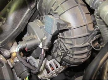
13. Unplug the wiring loom from the map sensor. Push down the clip at the top of the map sensor, then twist it anti clockwise and pull it away from the inlet manifold.
