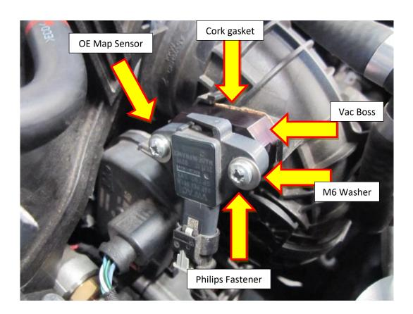
16. Push one end of the silicone vac hose onto the vac boss and secure it with a cable tie. Run the vac hose up to the dump valve and cut to length with scissors or a sharp knife. Use cable ties where there are arrows in the bottom picture.
