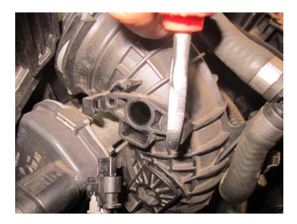
15. Re fit the Map sensor as shown in the picture below. First mount the cork gasket, next fit the vac boss (there is an arrow on the boss to show you which way should face up). The map sensor now fits on top of the boss and all three components are held in place with the two Philips head fasteners and M5 washers supplied.
