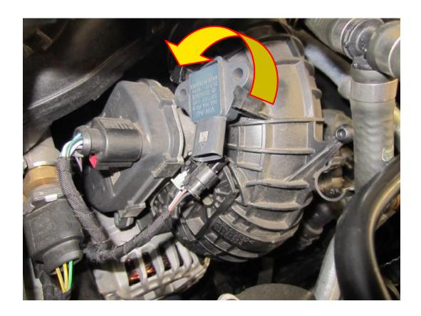
14. With the map sensor removed from the inlet manifold, the two retaining tabs shown in the below picture need to be removed. Use some side cutters or a junior hack saw to cut them off.
