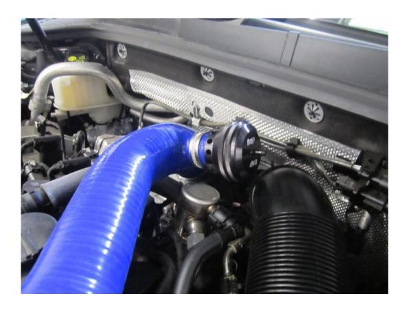
12. Locate the map sensor which you will find on the off-side of the inlet manifold.
