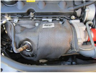
Please note that a turbo blanket will lose its flexibility over the first few heat cycles as the material cures, so once fitted it should <u>not</u> be routinely removed as this can cause damage to the blanket.
