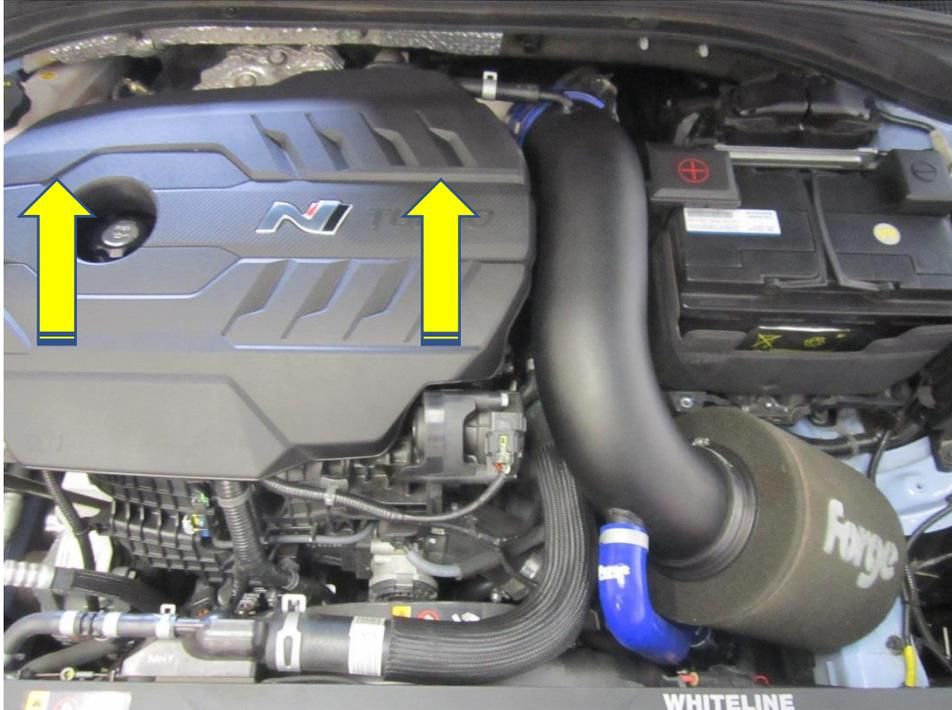
2. Using your hose clamp removal tool or long nose pliers remove the two breather hoses and dump valve recirculation hose from situ.
