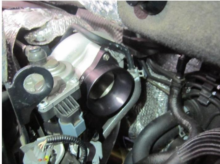
6. With the machined adaptor fitted to the turbo, you will be able to fit the Forge silicone inlet hose. Use the 70-90mm hose clamp provided to secure the inlet hose to the adaptor, fit it loosely at this stage to allow for adjustment.
