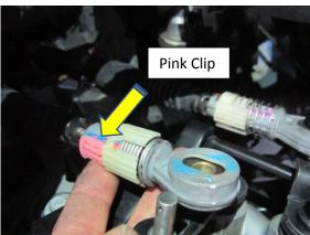
11. Tighten the three fasteners that hold the linkage to the gearbox, then test to see how the shift feels inside the car. If you think it needs adjustment this is the time to do so, now reassemble by following the steps 1-6 in reverse.
