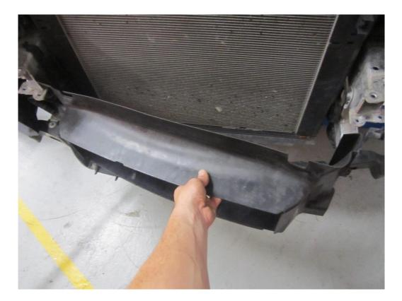
**16**. The lower bumper support is secured in place with two E11 fasteners, undo both fasteners and remove the support from the vehicle.
