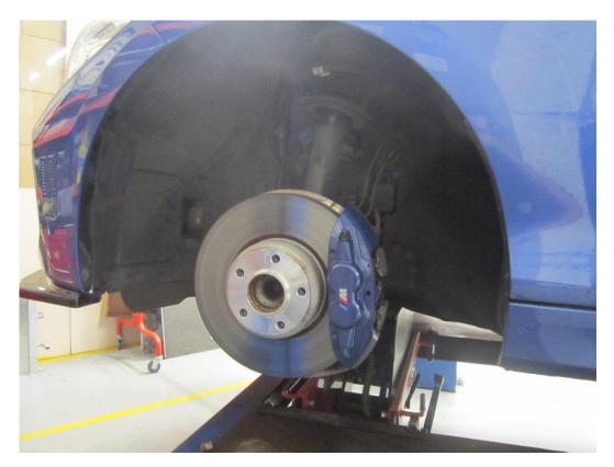
4. With the wheels removed, first locate all ten 8mm fasteners that hold the inner splash guard in place and remove them like before with the use of an 8mm socket and rachet or spanner. The splash guard will now pull away from the vehicle. This also needs to be repeated on the opposite side of the vehicle.
