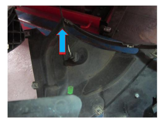
7. Remove the rubber seal that runs along the top of the bumper, with this removed it will reveal the six T30 fasteners that secure the top of the bumper to the vehicle. Use a T30 Torx driver/socket to undo and remove these fasteners. The bumper will now pull away from the vehicle.
