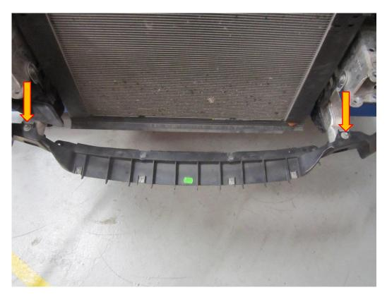
17. Undo and remove the two T27 Torx fasteners at the top of the radiator frame. There are two more T27 Torx fasteners at the bottom of the radiator frame on the underside, these also need removing, this bottom panel can be removed once you have un-clipped it from the coolant hose.
