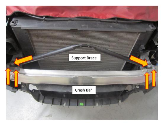
14. There are two plastic fasteners that hold the brake ducts which are either side of the radiators, remove these plastic fasteners with the use of a trim tool or flat blade screw driver.
