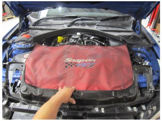
**11**. Remove the foam protector strip attached to the crash bar, this just unclips and pulls away from the vehicle.
