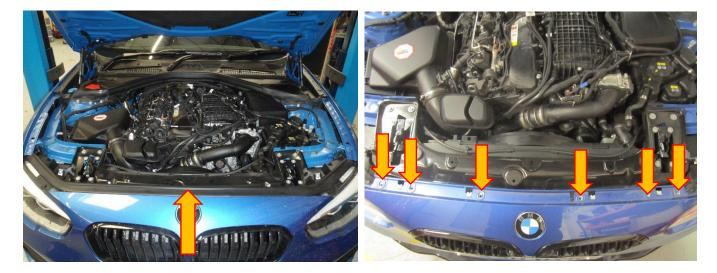
8. With the bumper off the vehicle you will need to remove the four T40 Torx fasteners located at the top of the slam panel, then remove the eight T30 Torx fasteners which secure the bonnet catches. Push the bonnet catches through the gap in the slam panel to make the removal of the panel easier.
