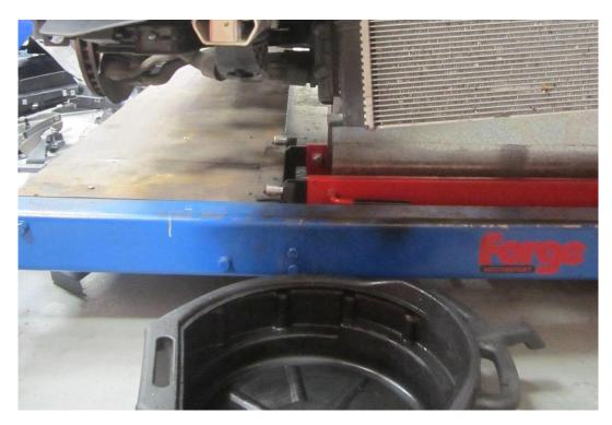
22. Use a flat blade screw driver to release the clip that holds the coolant hose coupler, now separate the coupler from the radiator and let the coolant drain into the drain pan below. When the coolant comes to a stop, release the coupler on the other side and remove the radiator from the vehicle.
