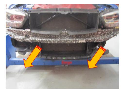
12. To remove the top air duct, first remove the rubber trim in the middle attached to the crash bar. There are two plastic fasteners that attach the duct to the crash bar, these can be removed by prising them off with a trim tool or flat blade screw driver. Finally, there are two tabs which hold the top ducting to the lower ducting, one each side. Push the tab outward to release it, now the duct can be removed from situ.
