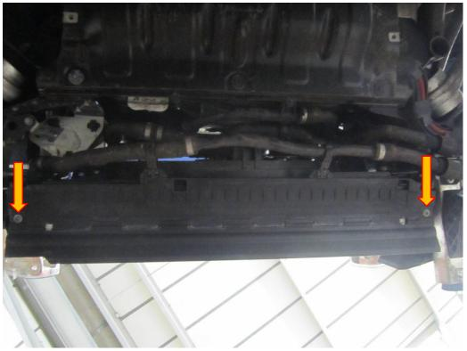
**18**. There are two T27 Torx fasteners that hold the whole radiator assembly to the vehicle, both need to be removed. You will now be able to lift the radiator assembly off the hook mounts.
