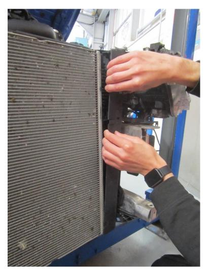
**20**. Remove the offside brake ducting, It is held in place with two plastic fasteners. Remove both fasteners to free the ducting from the vehicle.
