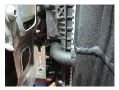
24. Make up the radiator frame by attaching the bottom panel to the side panels using the T27 fasteners removed earlier. Once the three parts are together position the pegs at the bottom of the Forge radiator with the mounting point at the bottom of the frame. Now push fit both sides of the frame and locate the
