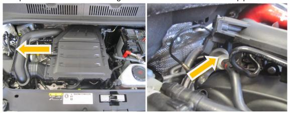
4. Unclip the couplers from the turbo inlet and throttle body while pulling them away from situ.
