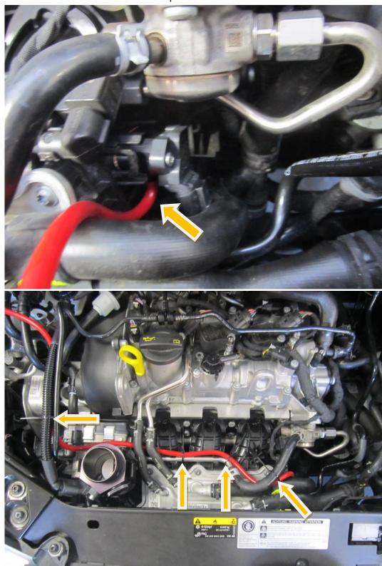
15. Prepare the silicone hose as shown in the picture below. Fit the valve to the hose and secure it with the provided hose clamp with the use a 7mm socket and rachet or a flat blade screw driver. Next, loosely place the two larger hose clamps at each end of the hose ready to secure the intake hose to the Forge motorsport billet couplers.
