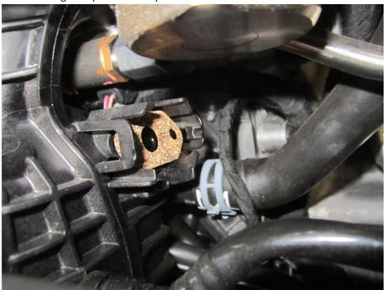
**13**. Fit the boost take off and map sensor into position and fasten with the M5x35 or M6X40mm screws provided.
