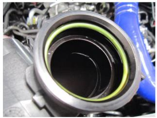
7. Remove the map sensor from the OEM boost pipe by prying the clips outwards and pulling the map sensor away from the housing.
