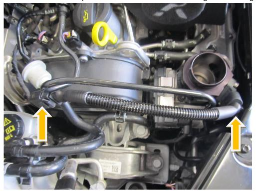
11. As pictured below remove the  $2^{nd}$  map sensor from the inlet manifold.
