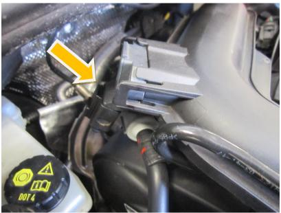
3. Unclip the vacuum hoses and wiring harness from the side of the boost pipe.
