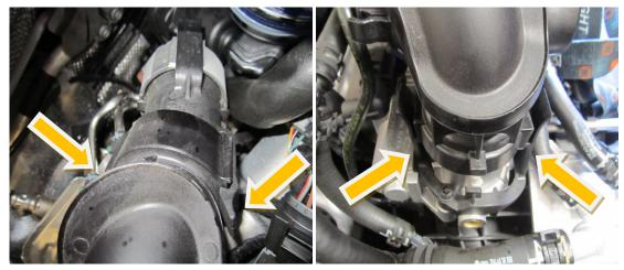
5. Remove the boost pipe fully from situ.
