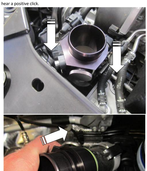
10. Plug in the wiring loom extension between the map sensor and the OEM wiring loom. With the cable ties provided in the kit secure the loom to the OE vacuum pipe, however leave this till step 13 and secure the loom and the Forge vac hose together.
