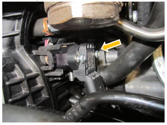
14. Fit the vacuum line from the dump valve to the boost/vacuum take off. Then cable tie the vac hose as shown in the second picture.
