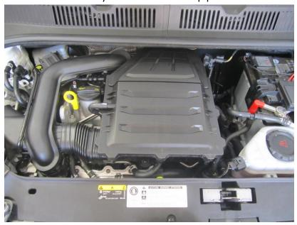
2. Unplug the wiring loom from the map sensor housed in the boost pipe.
