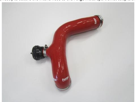
16. You will now be able to install the hose to the vehicle, simply push the hose onto the Forge motorsport coupler and secure with the hose clamp. Follow the same procedure at other end of the hose. Finally route the vacuum hose to the vac port on the end of the valve, cut off any excess length with a sharp knife then secure it in place with a cable tie provided.
