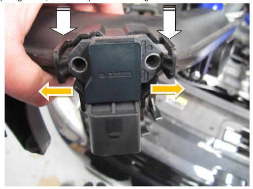
8. Fit the map sensor to the Forge motorsport billet coupler as shown in the picture below. Use the two M6x12 Allen cap fasteners provided to secure the map sensor, the blanking plug simply screws into the coupler in a clockwise direction.
