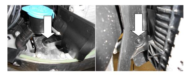
14. From inside the wheel arch using a flat blade screwdriver or similar tool remove the 2x clips. Pull the centre out first before removing the body of the clip.
