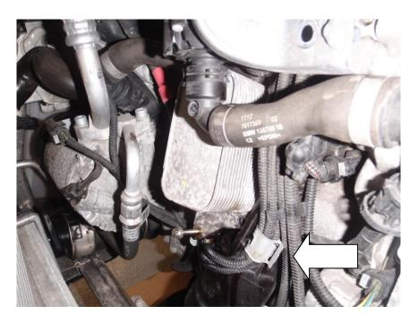
22. With the filter housing assembly removed from the car, using a T30 Torx driver, undo 4x remaining bolts around the perimeter of the water/oil heat exchanger.
