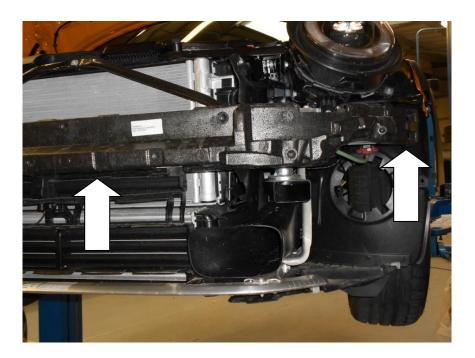
10. If fitted to your vehicle, unclip the wiring and using a T30 Torx driver undo the 2x bolts and remove the active air ducting. This part will not be refitted to the vehicle when the installation is complete.
