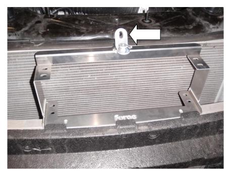
32. Using a scriber or marker pen mark the positions of the two holes in the base plate of the bracket on the crash bar.
