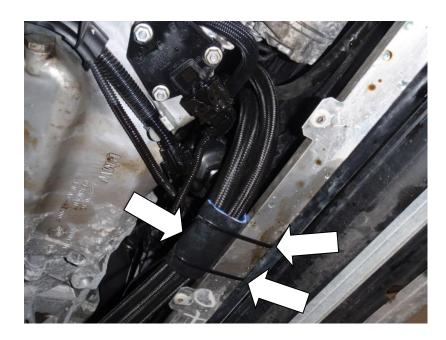
40. Use the remaining cable tie to tie the oil lines together just after the oil cooler.
