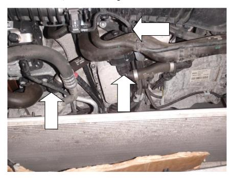
20. Using an E11 Torx socket and suitable ratchet undo the remaining 4 bolts.
