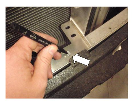
33. Using a 2mm drill bit, pilot drill a hole in the centre of the marked slots.
