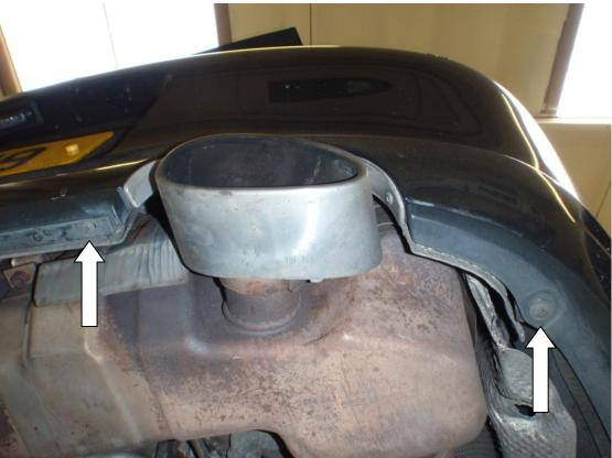
7. Now with the help of an assistant, tug the bumper rearwards off the plastic runners in the rear wings. When the bumper is pulled away enough, you will need to disconnect the electrical plug for the parking sensors and lights before removing the bumper completely and storing it somewhere safe.
