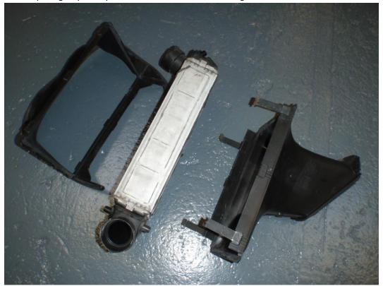
13. The new cores are slightly thicker so using a dremel or similar, you will need to remove plastic from both sides of the ducting as shown below, just leaving the vertical strips of plastic holding the clips on one side, and the clip receptacles on the other.
