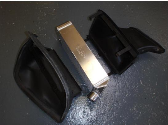
15. Line the threaded holes on the intercooler up with the rubber grommets on the frame. This time assembly is a little different – push the circlip onto the aluminium boss supplied FIRST, then place the washer under the circlip, then bolt the whole lot to the intercooler through the rubber grommet as shown below. You MUST use Loctite or a similar product in order to seal the threads as they protrude into the intercooler endtanks.
