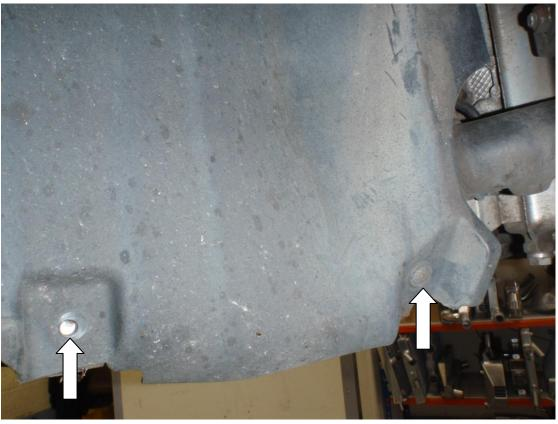
6. Now to fully release the bumper, remove the single torx and single Phillips head screw either side of exhaust pipe on each side.
