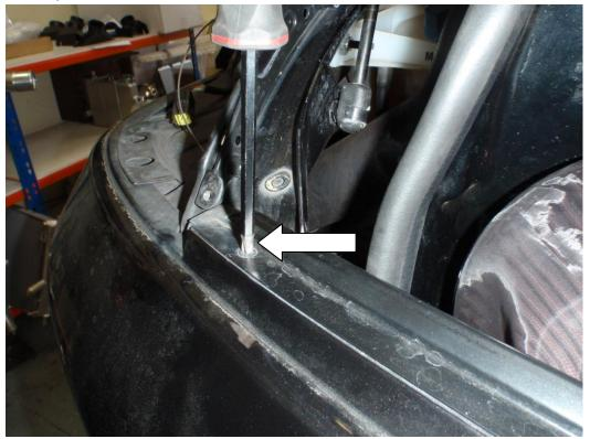
3. Working on the lower edge of each wheel arch, unto the two torx screws shown below.
