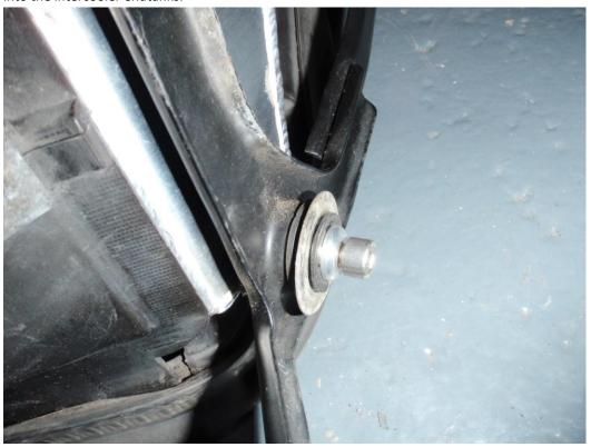
16. You will have noticed that the fourth grommet does not have a threaded boss in the intercooler – simply bend the unused grommet out of the way of the core.
