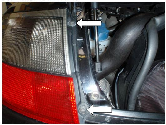
2. With both lights removed, undo the four Phillips head screws that hold the metal edging on the top of the bumper and remove from the car.
