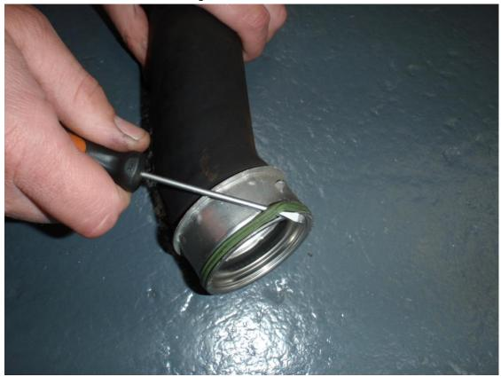
19. Place the rubber seals on the couplers provided, and push them securely into the crossover pipe in the engine bay until they securely 'click' into place.
