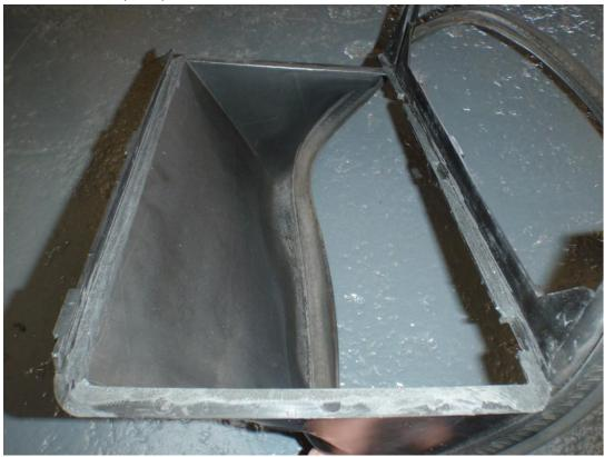
14. Of the two Forge intercoolers supplied, find the correct one for the side you are working on and reassemble it into the plastic ducting. Ensure that the ducting is central to the core as you fasten all the clips.
