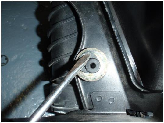
12. Unclip the upper and lower plastic ducting from the intercooler by pulling back on the end of the metal clips – again you may need a screwdriver as these are tight.
