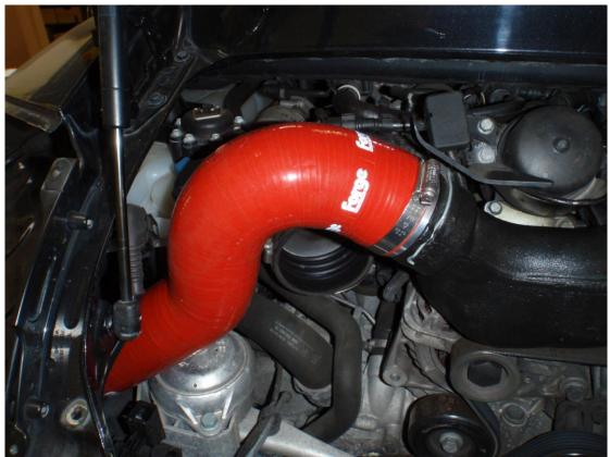
21. On the lower intercooler pipe, use the silicon hose supplied and secure with jubilee clips. The hose is subtlely different each side so they cannot be mixed up.
