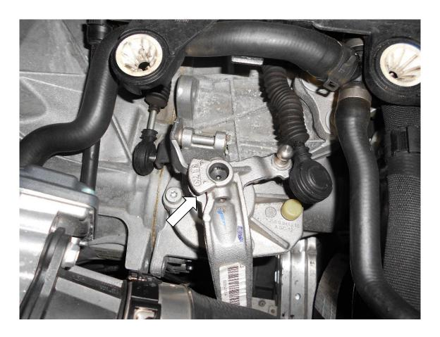
11. Using a 16mm spanner, tighten the adjustable ball in the required position. Closer to the selector shaft will give a shorter shift and further away will give a longer shift.
