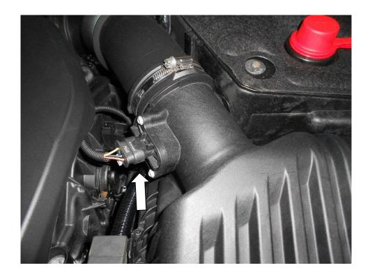
4. Using a 7mm Hose clamp driver or flat blade screwdriver loosen the hose clamp.
