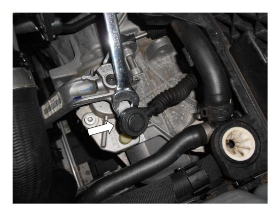
9. Place the Forge pin removal tool in position and using a 10mm Socket tighten the bolt to remove the locking pin.
