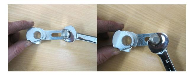
12. Prior to fitting the Forge quick shifter, make sure the selector shaft is clean and lubricated if possible. Secure the Forge quick shifter in position using the M6x40 allen cap head bolt and M6 nyloc nut provided. Ensure the up and down shift arm is correctly located.
