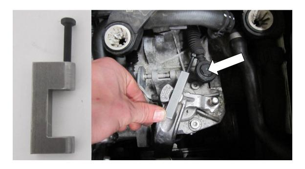
10. Carefully pull the shift arm upwards to remove it, a pulling tool is recommended for doing this if any corrosion has set in.
