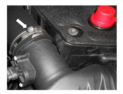
5. Using a 10mm socket, extension bar and suitable ratchet undo the bolt on the airbox bracket.
