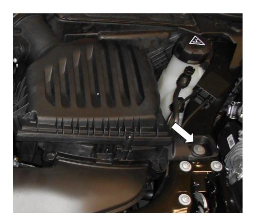
6. Pull the intake pipe away from the airbox pipework and firmly pull the airbox upward to release it.
