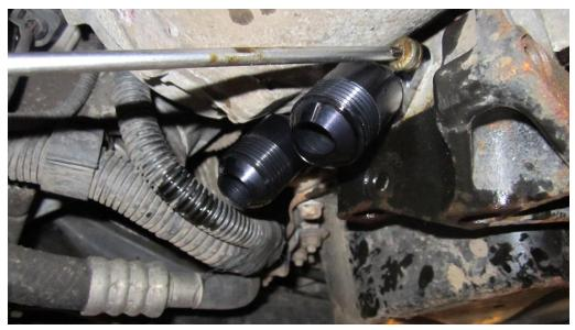
28. Slide your oil cooler assembly under and behind your crash bar into position.
