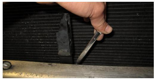
19. Now your fan control unit has been removed, place it onto your new Forge Motorsport bracket, using a 10mm spanner to tighten the 10mm nuts.
