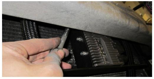
30. Now fix the upper two cotton reels on your power steering cooler to the lower part of your oil cooler bracket using the existing m6 nuts that were removed in section 13
