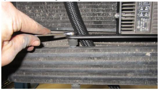
31. Feed your oil lines towards the left hand side of the vehicle when viewed from the front and through the slam panel towards the sandwich plate. Push the oil lines through where arrowed.
