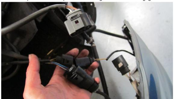
11. You also need to disconnect your washer jets, by pulling up the retainer and pulling out the hose. Have a jug ready to collect any screen wash you wish to keep.
