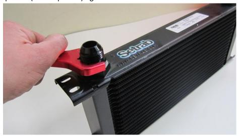
22. Find your oil cooler spacers and attach them to the oil cooler bracket using 4 M6 x 10 button heads and M6 washers provided, bolt up from underneath.
