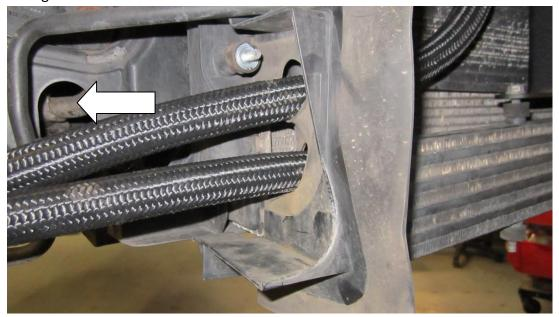
32. Connect your oil lines to the sandwich plate and tighten.
