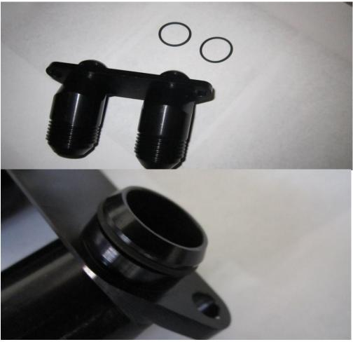
27. You can now install your sandwich plate to your engine. Put into position and use the two bolts you removed in section 12 to fix in place.
