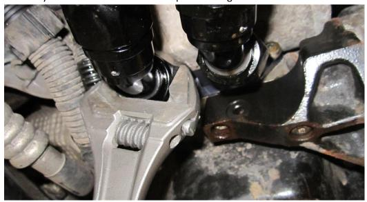
33. Slide the sandwich clamp into position hold the back plate in position and tighten the m5 countersunk provided with a 3mm Allen key.
