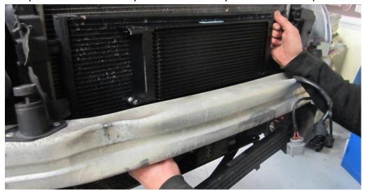
29. Using the two M6 hex heads removed in section 17 that held your fan controller bracket in position, attach your new assembly and tighten using a 10mm spanner.
