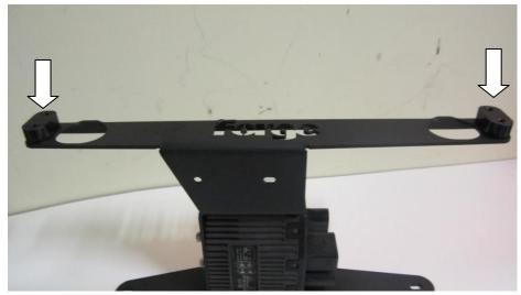
23. Now attach your new oil cooler again using 4 M6 x 10 button heads and washers.
