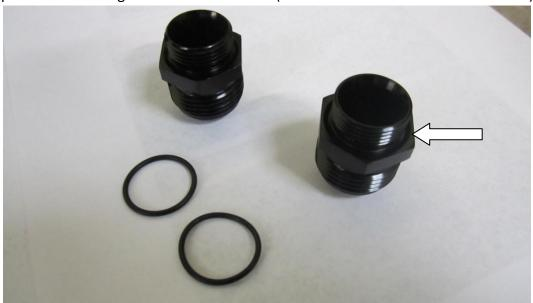
21. Now attach your M22 to dash 12 adaptor to your oil cooler, and using an adjustable spanner (or -12 spanner) tighten them down.
