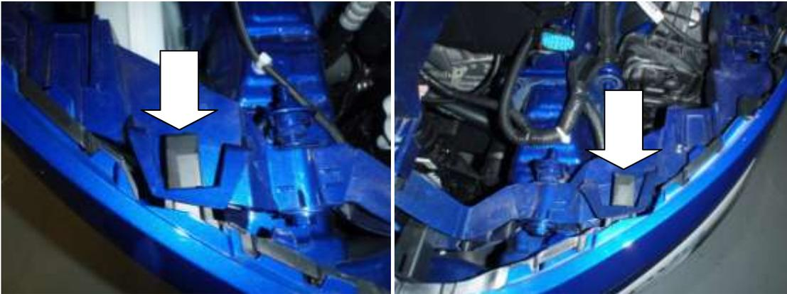
15. To remove the lower plastic air duct undo the 2x T30 Torxs and unclip from underneath.
