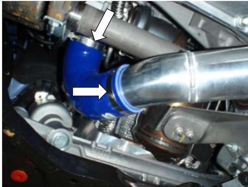
35. Use the remaining 90Deg silicone hose to connect the hard pipe to the intercooler outlet. Secure with suitable hose clamps.
