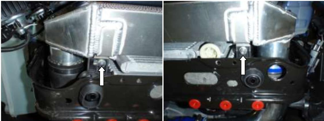
27. Once the intercooler is secured, use a 10mm socket to retighten the 2x bolts at either end of the radiator cradle.
