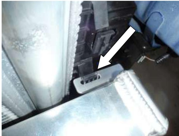
26. Using an M6X16mm Hex head bolt, 3x M6 washers and 2x M6 Nyloc nuts bolt the bottom mounts to original intercooler mounts.
