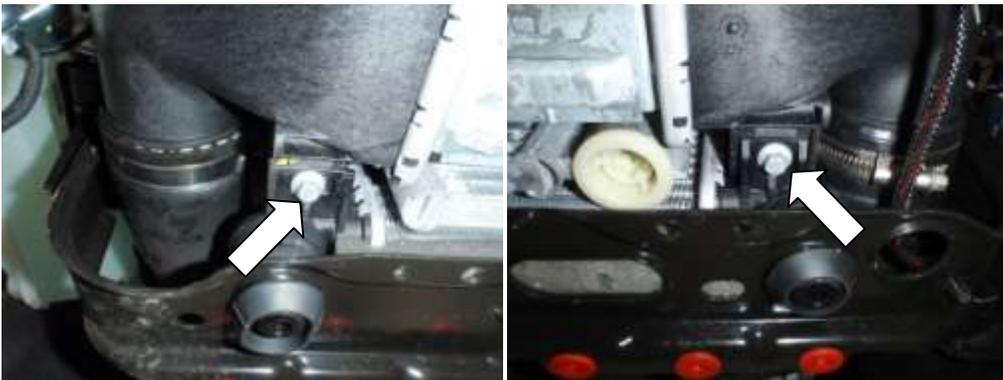
18. Using a 7mm Hose clamp driver or flat blade screwdriver undo the jubilee clips at either end of the intercooler and unclip the connector on the map sensor.
