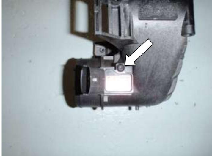
23. Using the M6x16mm Allen Head bolt and M6 washer bolt the MAP sensor to your new Forge Intercooler.
