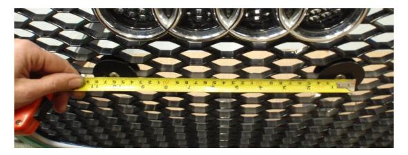
20. Using the button head bolts install the number plate.
