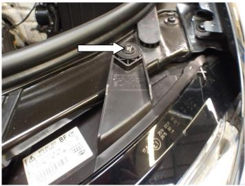
10. Unclip the head light washers and pull off the pipe.
