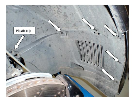
2. Undo the T25 torx screws under the front bumper and remove arch liner.
