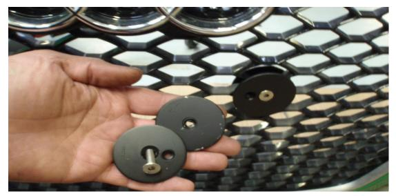
19. Measure between the new number plate fixings transfer onto the number plate. Drill new holes or move the disc's around until they match up with the existing holes.
