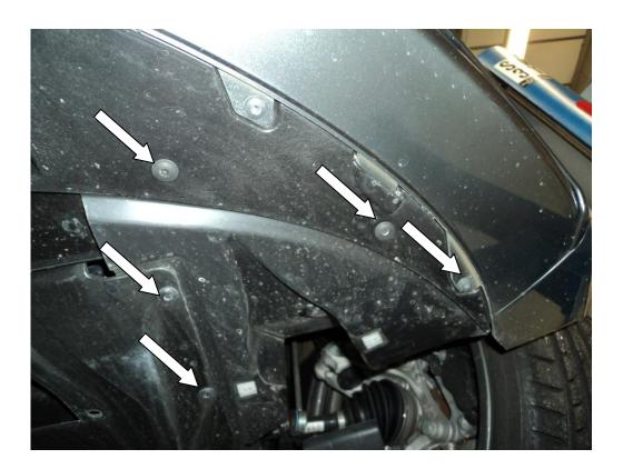
3. Undo the three T30 torx screws at the rear of the under tray, Undo the T25 torx screws from the front and sides and remove.
