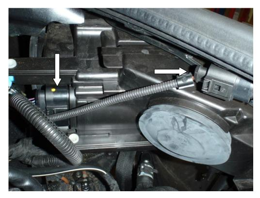
12. Unclip the headlight washer pipe work, undo the two bolts at each end and remove the crash bar. Instal the extra capasitey crash bar using the bolts just removed and reattach the washer pipe work.
