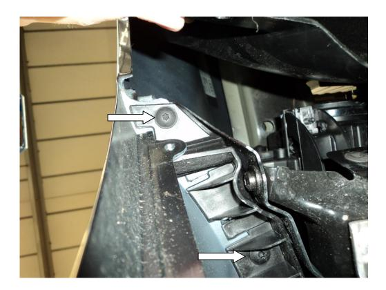
5. Remove the 13mm bolt from the back of the light this is hard to see and reach but you can excess from the inner arch.
