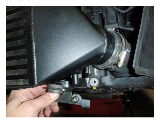
15. Now the intercooler is in the correct position lift up the washer pipe out of the way. Drill two holes with the drill bit supplied in the kit. Using the bolts from the OEM intercooler and the nuts and washers supplied attach the intercooler.
