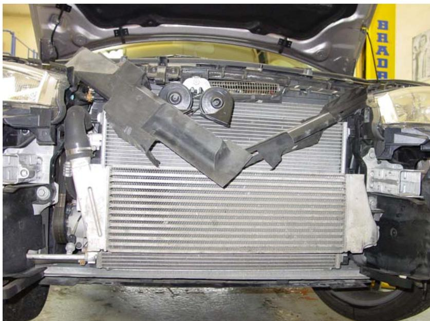
3/ Now fit the uprated intercooler in to place. Refit and tighten the 2 hose connections. You will now need to cut the plastic air diverters to suit the new intercooler shape; this can be done with a suitable sharp craft knife, hot knife or hacksaw. You can now refit the crash bar and complete bumper section in reversal of removal.
