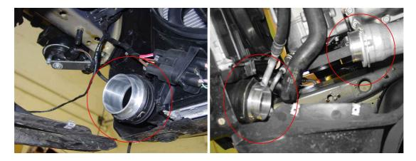
Remove the horns from their brackets and then remove each bracket from the car and refit the horns as per the pictures below with the new supplied brackets so they are now positioned higher. This is to allow extra space for the routing of the new hoses. If you do not wish to use the new supplied brackets, you may also just bend the OEM brackets to reposition the horns.
