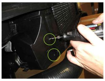
With the mounting holes drilled, position the Forge intercooler core in place and secure it using the supplied self-tapping screws and washers. If you encounter any resistance tightening the screws, please check the available depth of the hole to ensure that you are not touching the A/C condenser end tanks with the screws. Add washers as necessary if there is any conflict behind the holes.
