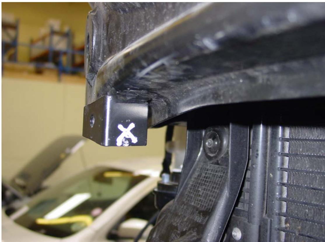
5/ Attach the brackets to the crash bar brackets as pictured below using the nuts and bolts supplied. Then mount the intercooler in to place also but only assemble the fixing nuts and bolts loosely at this stage.
