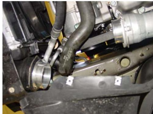
7/ Now fit the new hoses to join all the couplings and the new intercooler. The hoses may require a test fit to make sure they do not foul on any other engine or front panel components. A small amount of trimming may be required on the hoses at the new intercooler joints. Once you are satisfied with the fitment then secure all the hoses with the hose clips supplied.
