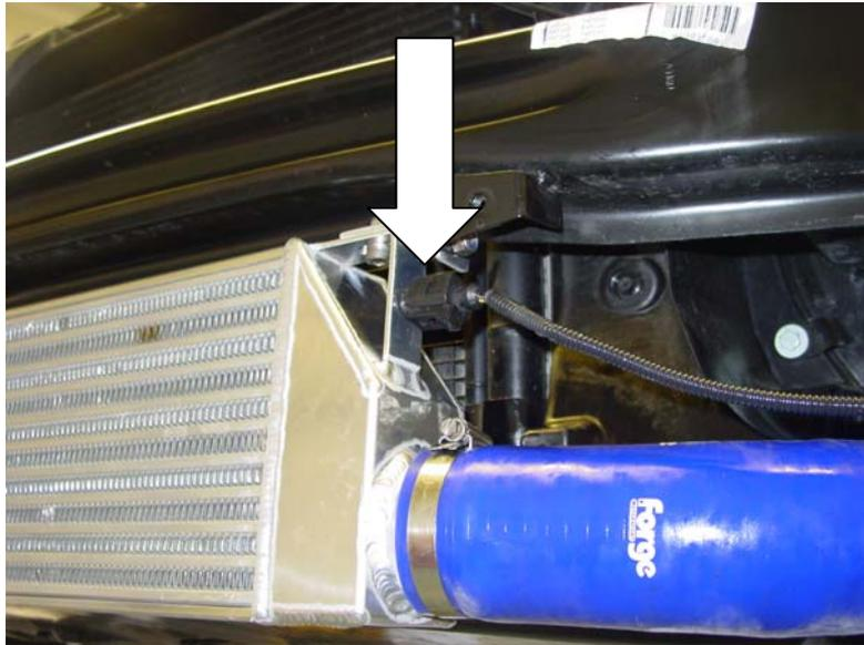
9/ Before the bumper can be refitted you have to remove the lower plastic brace panel as shown below. This can be simply removed from its plastic fixings with a sharp knife and a drill. You may also need to remove the two plastic prongs on the edge of the foglight covers nearest the intercooler as they can foul the intercooler hoses on certain models.
