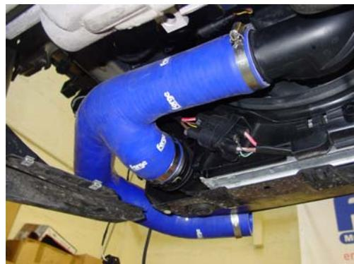
8/ Now centralise and tighten the fixing bolts on the intercooler. Fit the ambient temperature sensor as indicated below.
