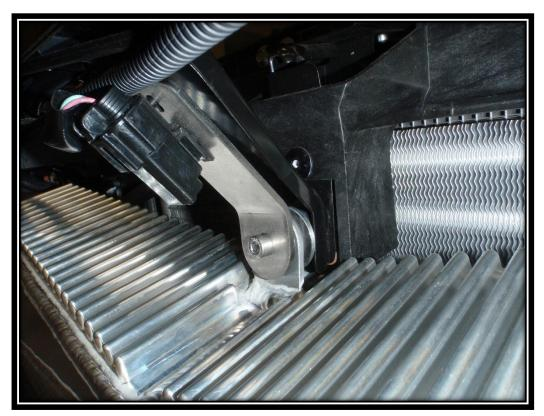
10. Fit the rubber grommets and small aluminium inserts into the brackets.
