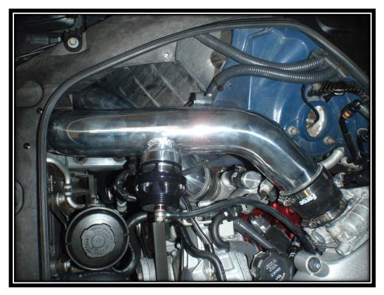
24. Make sure the dump valves are level and down far enough to clear the bonnet and tighten jubilee clips.
