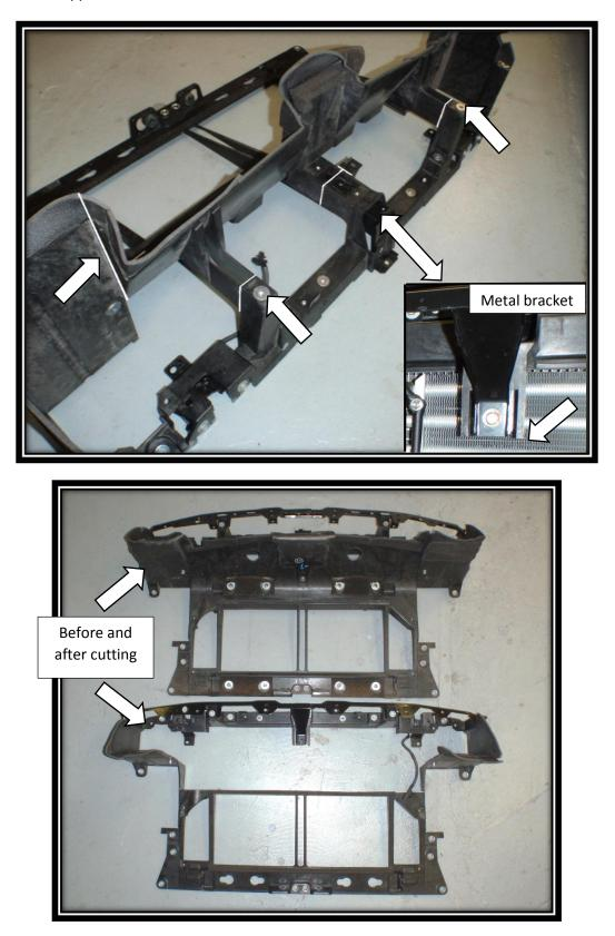
3. Mark the cutting line on the middle support at the bottom of the metal bracket. The two side supports need to be cut flush at the bottom.
