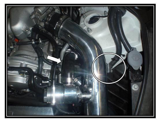
26. The inlets of the intercooler have bosses for installing Forge Motorsports IPCV and valves. However they could be used for boost readings etc. or just blank the off using the short button head bolts provided.
