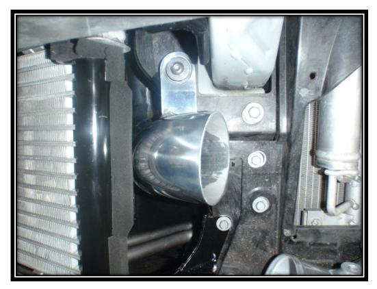
17. Loosely fit the silicon hose to the turbo on the oil cooler side, you will notice it fits up against the oil cooler bracket mark around the silicon hose and grind the bracket away for clearance.
