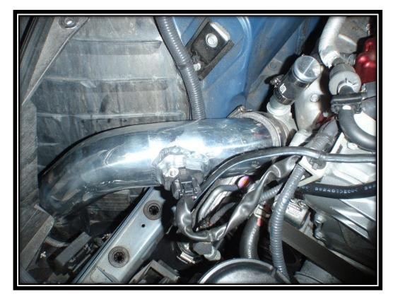
21. Install the silicon hoses to the top of the intercooler loosely with the clips in the position as shown below.
