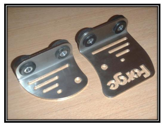
11. Refit the crash bar, bolt the brackets to the intercooler then attach the brackets to the crash bar using the self-tapping screws and large washers supplied with the kit. Please note the crash is an optional extra.
