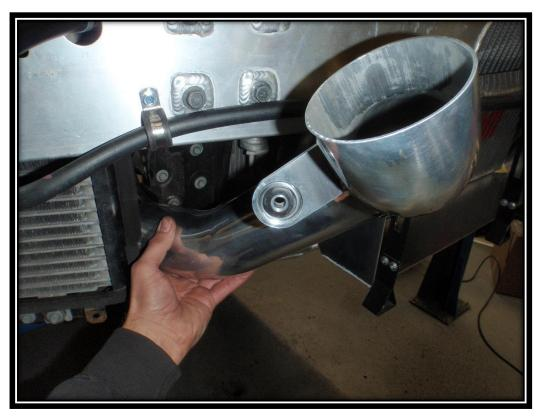
16. Bolt in the induction pipes with the long M8 button head bolts and large washers, and tighten the silicon hose onto the inlet pipe in the engine bay.
