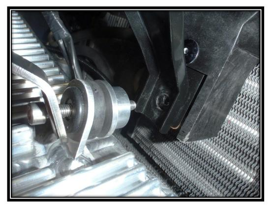
9. New position of air temperature sensor.
