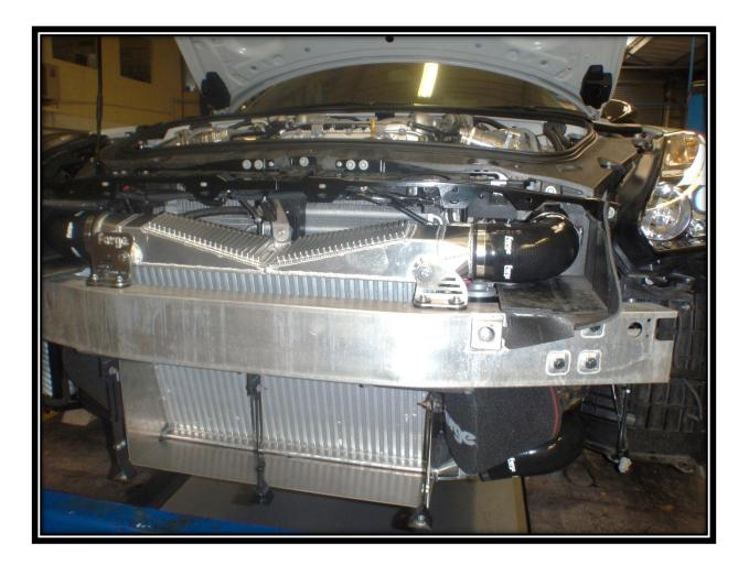
1. Remove the front of your vehicle plus all the intakes and boost pipes. Please refer to the forge motorsport strip down instructions if you have not done this before.
