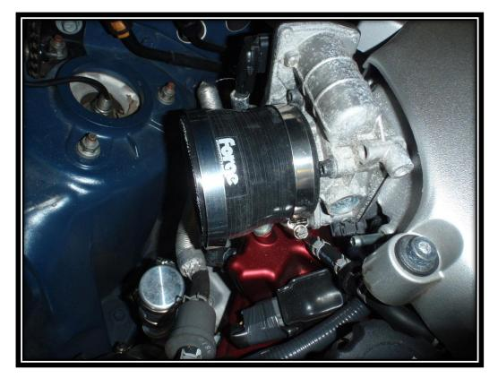
23. Install the dump valves onto the top boost pipes so they can be positioned correctly when the boost pipes are fitted. Fit the boost pipe into the intercooler silicon hoses, push into the silicon hose as far as possible then rotate and push into the throttle body.
