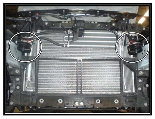
5. Plug in horn wiring extensions and bolt the horn where the metal intake shield would have fitted.
