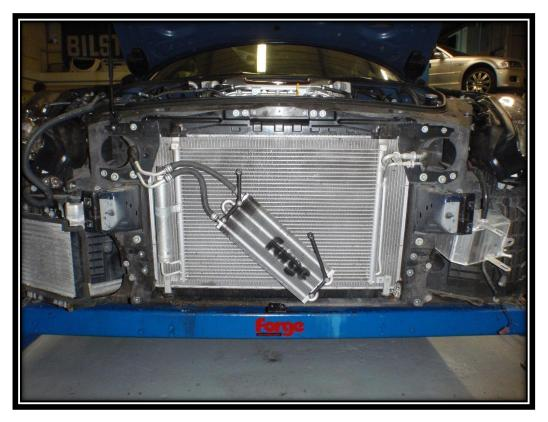
2. Mark out the radiator pack/ducting just above the foam or rubber strip, as shown below.
