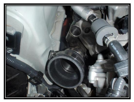
13. Remove the M8 bolt as shown below on both sides.
