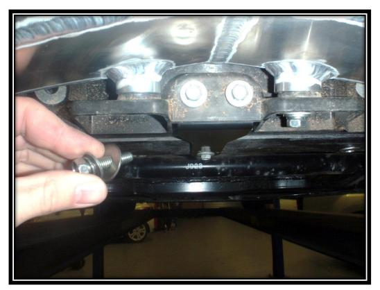
8. Holding the intercooler in position place the long M6 bolt supplied through the air temperature sensor bracket, through the rubber grommet and aluminium top hat spacer.
