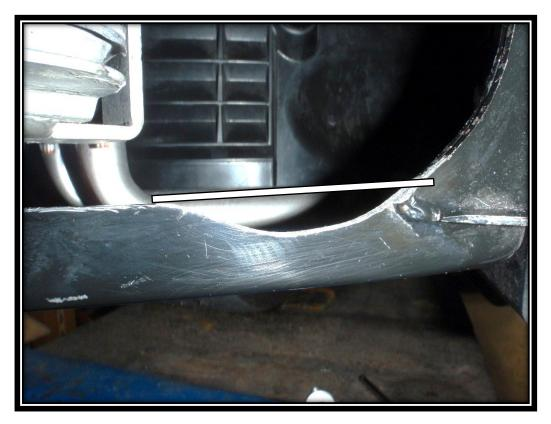
18. Now install the lower silicon boost hoses and tighten making sure there is enough clearance between the silicon hose and the bracket.
