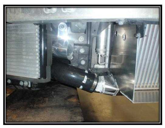
19. Install the filters so there is approximately a 10mm gap between the filter and intercooler.
