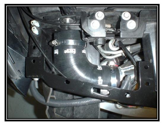
22. Install the silicon hoses to the throttle bodies loosely with the clips in the position as shown below.
