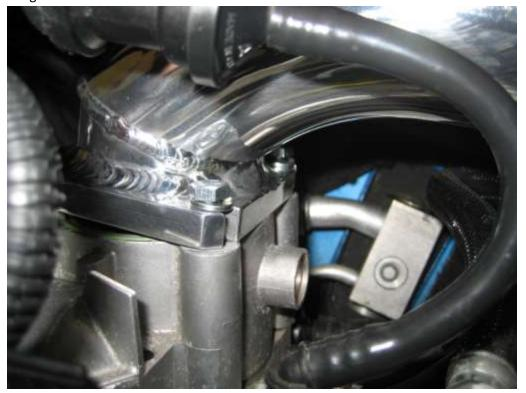
35. Use the last bracket and connect it to the rigid airbox pipework using the nut and rubber damper you saved from step 32, together with an M6 nut and washer, and orientate the bracket so that the other end locates over the front right bolt on the throttle body.
