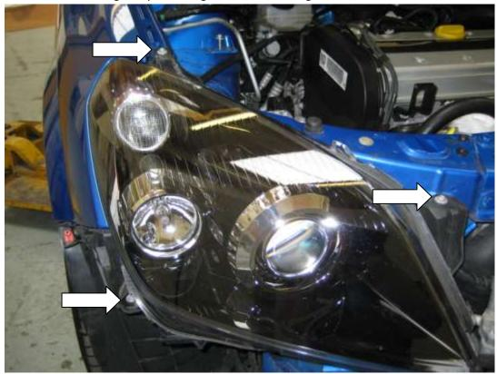
...then remove the wiring at the rear of the headlight unit by tilting it forward, and inserting a screwdriver into the red section of the connector and prising it outward to release the clip. Remove the headlights and store somewhere safe.
