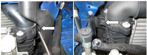
19. Lift the intercooler slightly to release the bottom right clip from the radiator
