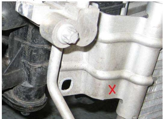
22. Drill the top right mount where the intercooler fitted to the radiator with a 5mm drill bit (no bigger), and use one of the supplied st/st self tapping screws in this location to remount the condenser to the car using the two supplied Forge brackets and the bolts you removed in section 17. Use the new hole you drilled for the lower left mount. The new brackets should push the condenser back against the radiator, and slightly to the left.
