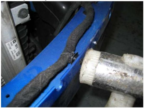
13. Undo the four long bolts that pass through the crash bar (two each end) with an E14 socket on the top and 13mm spanner on the bottom. On the passenger side, also undo the 13mm bolt holding the washer bottle to the crash bar.
