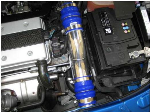
34. Screw in two M6x80mm with spring washers on the two right hand bolt holes of the throttle body, so they are about 15mm from being screwed down fully. Push the flange of the last aluminium pipe under the bolt heads and washers through the cutouts in the side of the flange.
