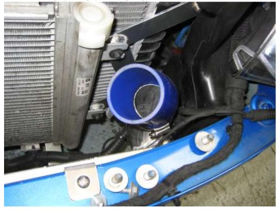
30. Put the supplied 90 degree bend with tag welded on the side into the silicon hose, and align the tag so that you can loosely screw in the bolt under the slam panel removed in step 11.
