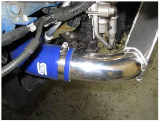
29. On the exit of the intercooler, place the longer leg of the supplied 45 degree silicon elbow so that the short leg is pointing up at an angle, again with clips to suit.
