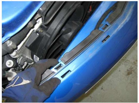
7. If headlight washers are fitted, place a bucket under the washer bottle and squeeze the fitting on the hose attached to the bumper to remove it. Remove the air temperature sensor wiring from the back of the bumper grille. The bumper can now be withdrawn from the car while the washer bottle empties.
