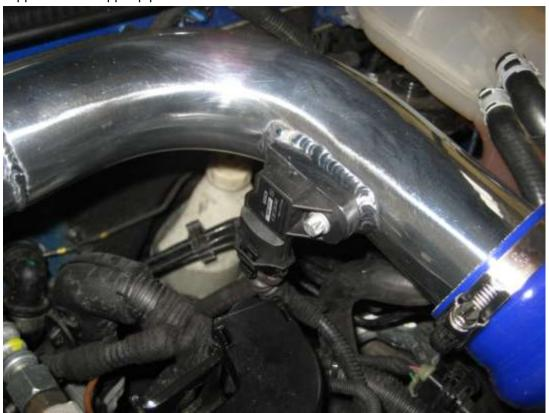
37. Move the pipes around until you have approx 25mm of aluminium in each end of the silicon joiners, then tighten up all the hose clamps and the bolt under the slam panel.
