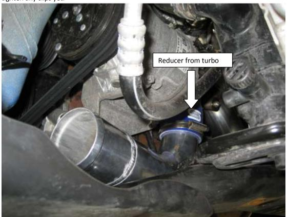
28. Onto the end of the aluminium pipe, use a 90 degree silicon bend and suitable clips, and connect the other end to the inlet on the intercooler. When everything fits, and the aluminium tubes are all approx 25mm inside the silicon hoses, tighten all hoses with a 7mm hose clamp driver or socket.
