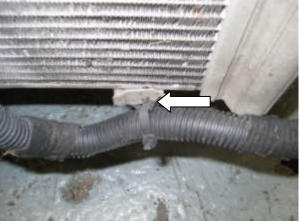
16. Remove the two 13mm nuts holding the top edge of the condenser fan to the condenser, and lift up to remove the fan. There should be enough slack in the wiring to allow you to place the fan on the floor in front of the car.
