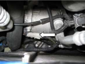
15. Pull the wiring loom around the condenser, and unclip from the bottom of the condenser on the drivers side and the front edge of the condenser (two clips) on the passenger side.
