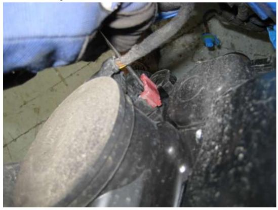
10. Undo the three 13mm bolts on each end of the slam panel (you may need to remove the single 10mm bolt holding the top of the washer bottle for access).
