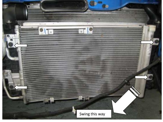
18. Undo the top left and top right screw holding the stock intercooler to the radiator.
