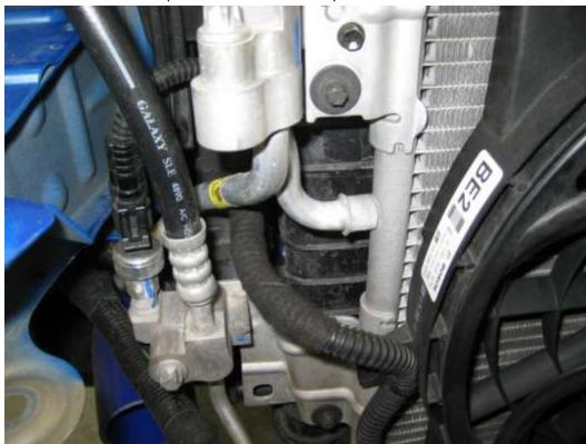
24. Remount the crash bar to the car using the nuts and bolts removed in step 13, clip the wire back in and then drill out the two prexisting 4mm holes on the top face of the crash bar to 5mm – NO MORE.
