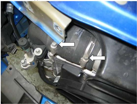
...undo the retaining bolt holding the pipe to the top of the radiator on the passenger side, then undo the hose connecting to the turbo and remove the whole pipe run from the car.
