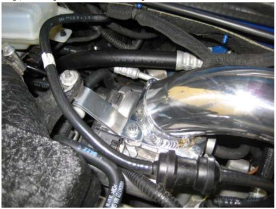
36. Retrieve the MAP sensor and screw you removed in step 31 and screw it to the boss supplied on the upper pipe. Reconnect the electrical connector.
