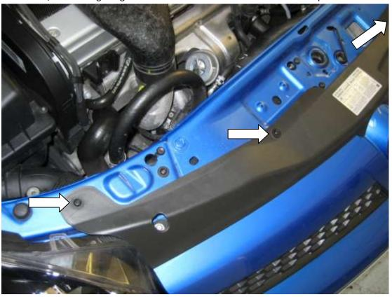
2. Remove the two T20 screws in each wheel arch
