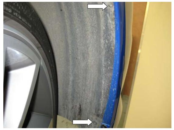
3. Working under the car, remove the three fixings that hold the undertray to the chassis by prying out the central peg to loosen it and then removing the whole fixing.
