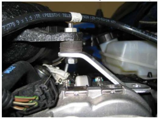
Bolt the remaining two M6x80 bolts and spring washers through the left hand holes in the flange, and through the bracket at the front. Tighten all the bolts down.
