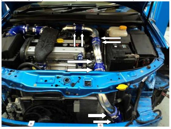
38. Locate the wiring for the air temp sensor you removed in step 7 and pull it over the top of the intercooler to leave it in front. Reattach the plastic and foam bumper supports removed in step 4. On the back of the bumper, if headlight washer are fitted, locate the short length of hose that connects to the washer bottle, and remove it from the tee piece. Remove the connector by slicing the hose.
