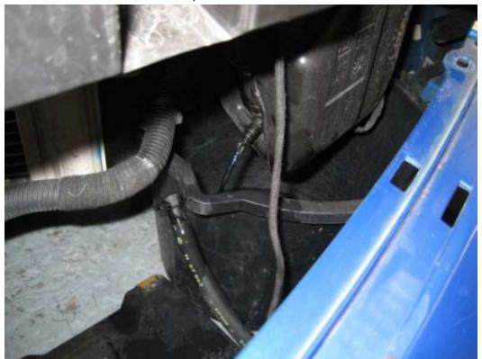
8. Remove both foam pieces from the ends of the crash bar (they just lift off), and drill out the two rivets with a 4mm drill bit to remove the plastic bumper reinforcement.
