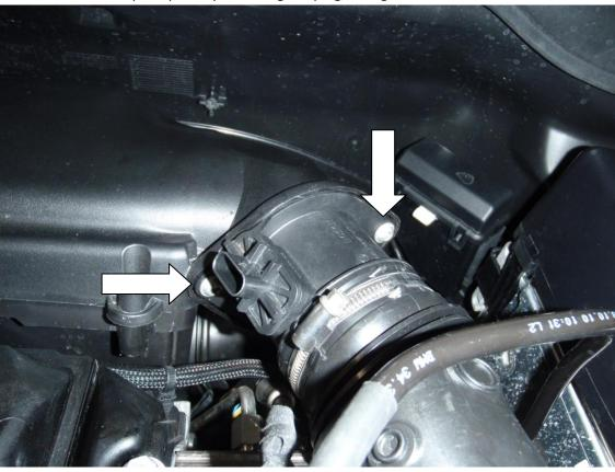
2. Undo the T25 Torx bolt holding the air filter down.
