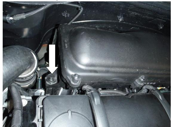
3. Now pull the air box upwards to release it from the rubber lugs.
