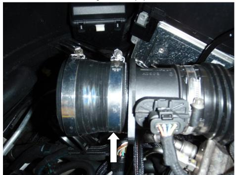
6. Fit the air filter to one end of the alloy pipe, and then the alloy pipe to the reducing silicon hose. Then using the self tapper provided, screw that into the slam panel, tightening the 2 hose clamps.
