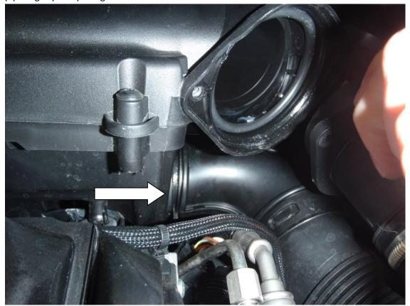
5. Fit the silicon hose reducer using the hose clips provided, to the air mass sensor.
