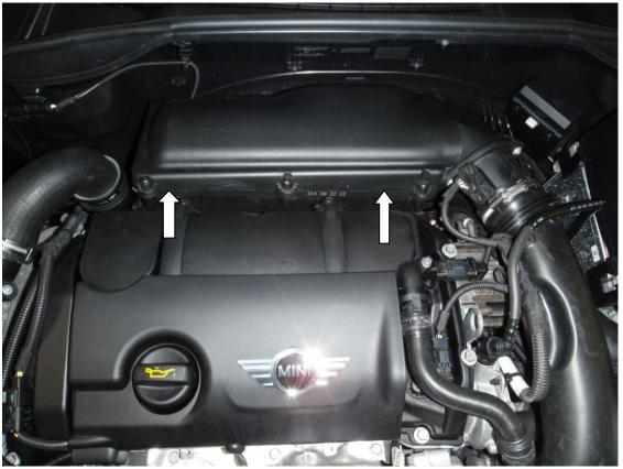
4. Remove the cold air feed that connects to the bottom of the air box by simply twisting the pipe slightly and pulling outwards. Now the air box can be removed.
