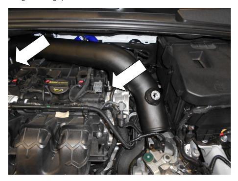
17. Carefully twist and remove the sensor from the OEM airbox.
