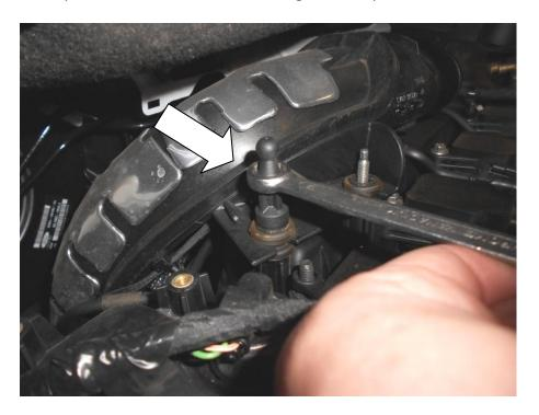
11. Undo the 8mm bolt on the second hard pipe and remove it.
