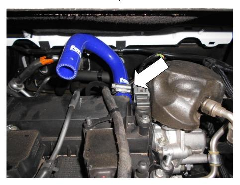
15. Place the 63/76mm silicone reducer on the turbo inlet and secure with a suitable hose clamp.
