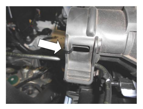
7. Using a 7mm hose clamp driver undo the hose clamp on the turbo outlet, located at the back of the engine. (Photo taken from underneath the vehicle to illustrate)
