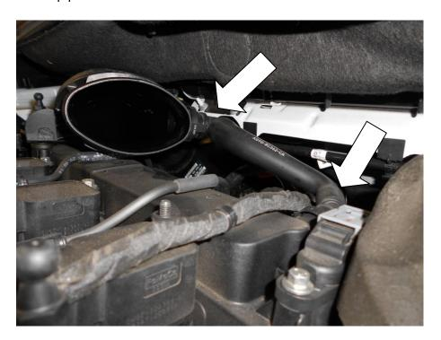
13. Remove the final part of the OEM induction pipework.
