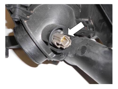
18. Insert the sensor in your Forge hardpipe, twist the senor until it stops against the raised tab.
