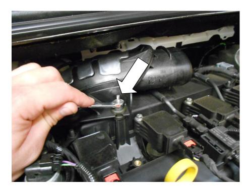
10. Using a 12mm spanner undo and remove the engine cover pin.
