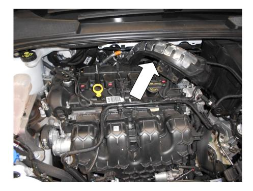
14. From your Forge Induction kit join the 19mm 180deg silicone hose to the cam cover breather and secure with a 25mm hose clamp.
