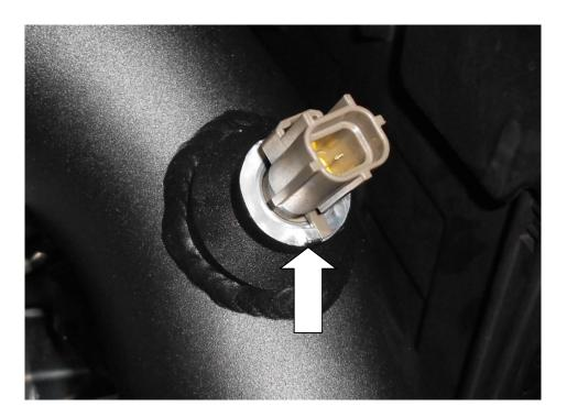
19. Reconnect the wiring to the sensor.
