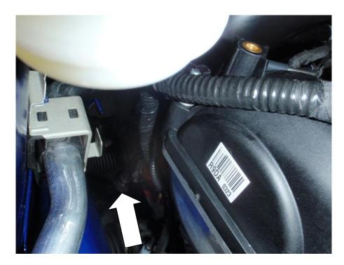
16. Place your Forge Induction pipe in position, connect the 19mm outlet to the open end of the silicone hose running from the cam cover, secure with a 25mm hose clamp. Bolt in place using the fixings provided.
