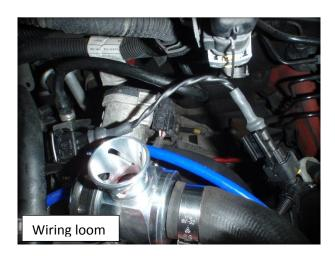
10. Attach the short silicon hose and blanking plug to the filter pipe.
