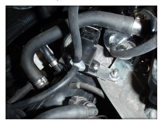
8. Attach the BOV with the P clip supplied in the kit to the bottom right bolt where the stock valve used to be fitted. Using the hose clip reattach the hose and bolt down the breather assembly.
