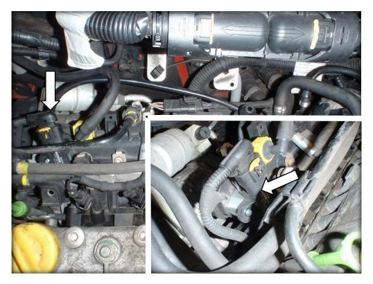
7. Attach the solenoid to the top left bolt where the stock valve used to be fitted.
