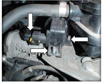
5. Undo the bolt from the MAP sensor on the metal boost pipe and fit the spacer block with the vacuum pipe pointing to 3 o'clock. Reattach using the 30mm long M6 bolt and small washer supplied.
