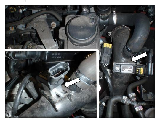
6. Undo the bolt from the MAP sensor on the inlet manifold and fit the spacer block with the vacuum pipe pointing to 12 o'clock. Reattach using the long screw with a Philips head supplied.
