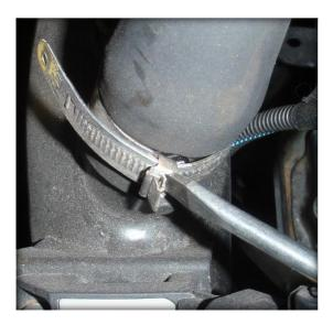
3. Remove the clip from the bottom part of the stock valve, undo the three bolts on the breather assembly and rotate to gain excess to the stock valve.
