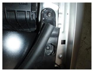
You now need to attach the two inlet ducts. The side duct is secured using the two T30 Torx screws that secure the upper edge of the radiator support just behind the headlight.
