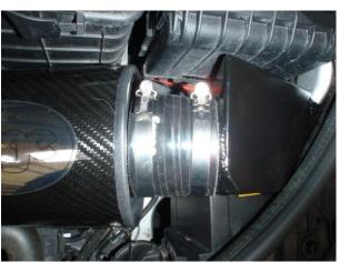
You may find it easy to attach one of the carbon filter canisters at the same time, using a 76-70 straight coupler hose to attach the opposite end of the filter canister to side inlet duct, securing it with a #90 and #80 hose clamp. NOTE: During installation, the filter canisters should be oriented so that the the open end of the filter is attached to the pipework going to the throttle body and the pointed end of the filter is attached to the inlet duct.
