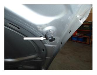
When closing the bonnet/ hood for the first time, check the level of the panel against the wing / fender edge. If necessary adjustment can be made with the adjusters found on the underside of the bonnet / hood as indicated.
