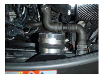
The forward facing ram-air duct is now attached to the front radiator support / slam panel using the original T25 Torx screws that secured the original intake ducting that were removed previously.
