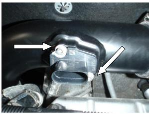
Remove front air duct securing fasteners. There are three fasteners ( arrowed ) to remove on the battery side of the duct and one fastener on the engine side.
