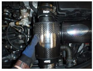
You can now attach the second carbon canister using the remaining two 76-70 straight couplers. Due to the fixed nature of the pipe and the forward ram-air inlet duct, it will take some effort and maneuvering to insert the canister and attach both couplers to the piping. Once both couplers are attached to the piping, however, secure the hose clamps.
