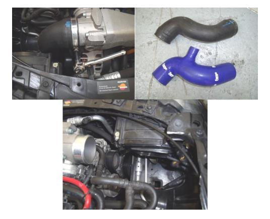
• Fit the relocation hose with the spout closest to the throttle body using the hose clips supplied.
