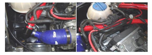
Next connect the megaflex to the turbo intake pipe where the dump valve was originally located using the plastic 90
