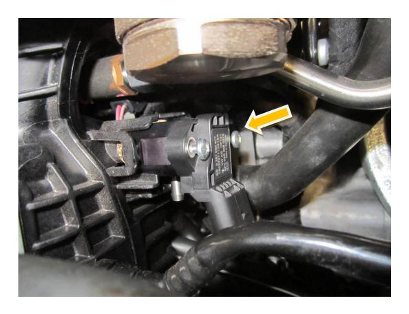
14. Fit the vacuum line from the dump valve to the boost/vacuum take off. Then cable tie the vac hose as shown in the second picture.
