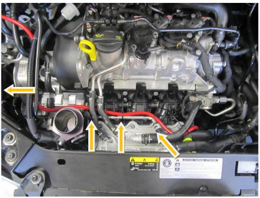
15. Prepare the silicone hose as shown in the picture below. Fit the valve to the hose and secure it with the provided hose clamp using a 7mm socket and rachet or a flat blade screw driver. Next, loosely place the two larger hose clamps at each end of the hose ready to secure the intake hose to the Forge Motorsport billet couplers.
