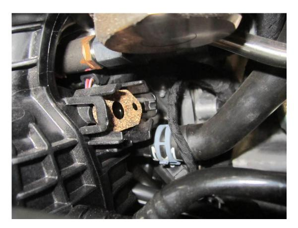
**13**. Fit the boost take off and map sensor into position and fasten with the M5x35 or M6X40 screws provided.
