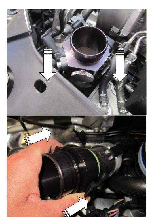
10. Plug in the wiring loom extension between the map sensor and the OEM wiring loom. With the cable ties provided in the kit secure the loom to the OE vacuum pipe, however leave this until step 13 and secure the loom and the Forge vacuum hose together.
