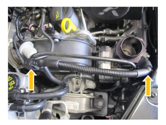
11. As pictured below remove the 2<sup>nd</sup> map sensor from the inlet manifold.
