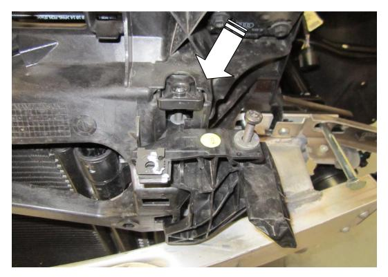
25. Disconnect the wiring loom plugs shown in pictures below. This is to enable you to remove the condensor radiator and intercooler pack with ease .
