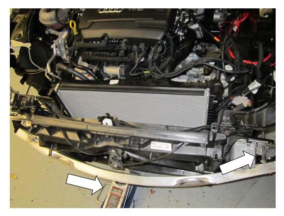
30. Remove this part of the plastic cowling where the air condensor pipes pass through the intercooler assembly housing by pushing in on the tabs as arrowed .
