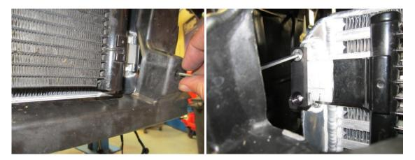
39. Please study the photos below to see where to drill the access holes in order to tighten some of the mounting clamps. The mounting clamp closest to the condensor pipes can only have one of the fasteners tightened dont worry as the cowling itself will hold this in position when fully installed.
