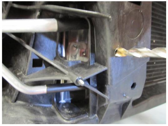
40. Place the rubber O-rings provided over the mounting clips on the radiator.
