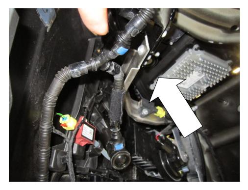
15. Using a flat bladed screwdriver prise up the clips that hold on the front bumper, these are beneath the torx fasteners you removed in section 12. To make it easier a second person should help you lift and remove the bumper safely without damaging it , however this can be done alone.
