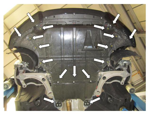
8. Using the T20 torx drive remove the fasteners that bolt the bumper to the wing on both sides of the vehicle. Once these have been removed pull the lower bumper away from the arch to unclip the bumper ready for removal .
