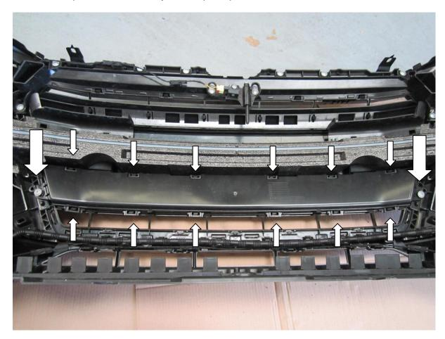
17. Undo the T30 fastener that holds the under light brace bar .
