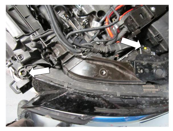
22. Undo the three T30 torx screws underneath the headlight next to the wing.
