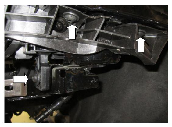
23. Next remove this tab light mechanism from the top of the headlight. Now slide the headlight out from under the housing.
