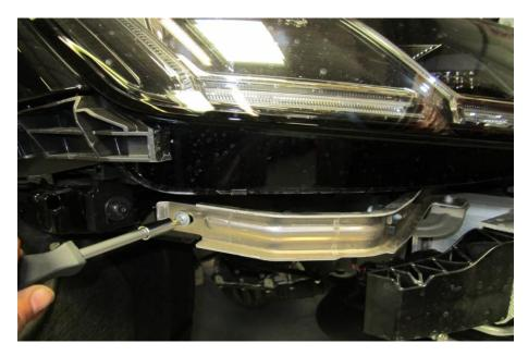
18. Undo the two T30 Torx fasteners above each headlight .
