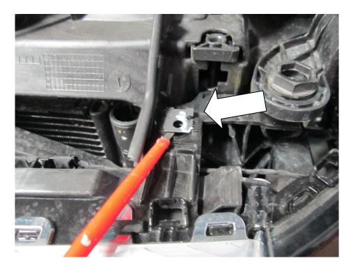
16. Now the bumper is off you can remove a part of the plastic grill. This does nothing but restrict air to your vehicles cooling systems. Your intercooler and radiator will benefit from the removal of this part. Using a T20 torx drive remove the two fasteners arrowed in the picture below then just unclip the plastic cover and remove .
