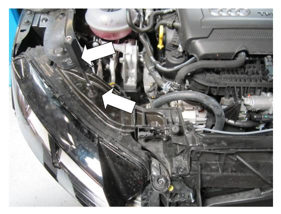
19. Disconnect the air temp sensor and remove the ducting either side of the intercooler assembly.
