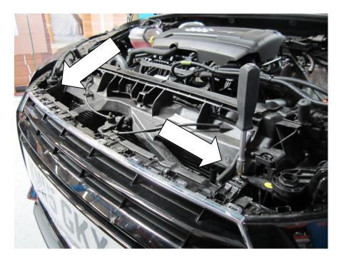
14. Undo the front light washer jet, this can be found behind the front bumper on the passenger side (RHD vehicles).
