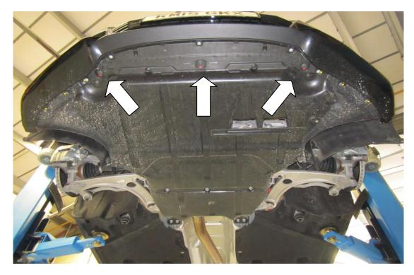
7. Now using the T20 and T45 Torx drives remove the fasteners pictured ,there are also two trim clips at the rear of the undertray that must be removed.
