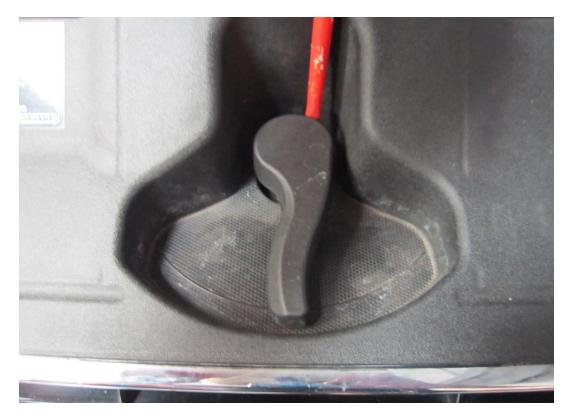
12. You will now be able to remove the plastic panel underneath the lever, pull in an upwards motion to remove.
