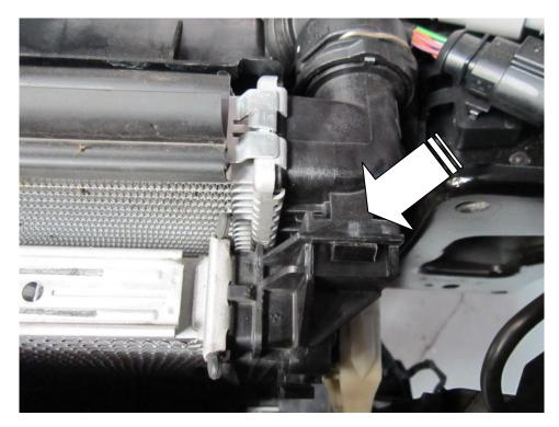
32. Remove the rubber ducting which sits either side of the condensor, This will no longer be used as your Forge Motorsport intercooler is a lot thicker than your OEM item.
