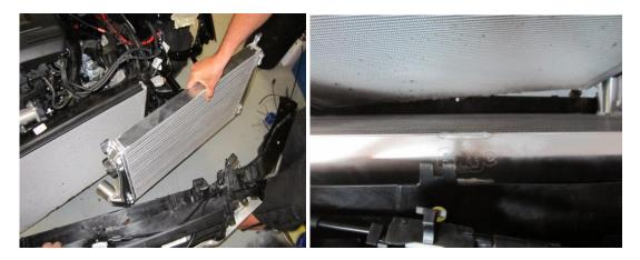
38. With the new intercooler in place fit the condensor into the mounting position then using a 3mm allen key fasten the mounting plates in place. You will need a drill and a 5 mm drill bit to drill some holes in the plastic cowling to access some of the fasteners.
