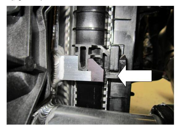
42. Before clicking the radiator into position remove the plastic cover that is mounted on top and push the radiator into the rear of the intercooler making sure the tabs are fully inserted.
