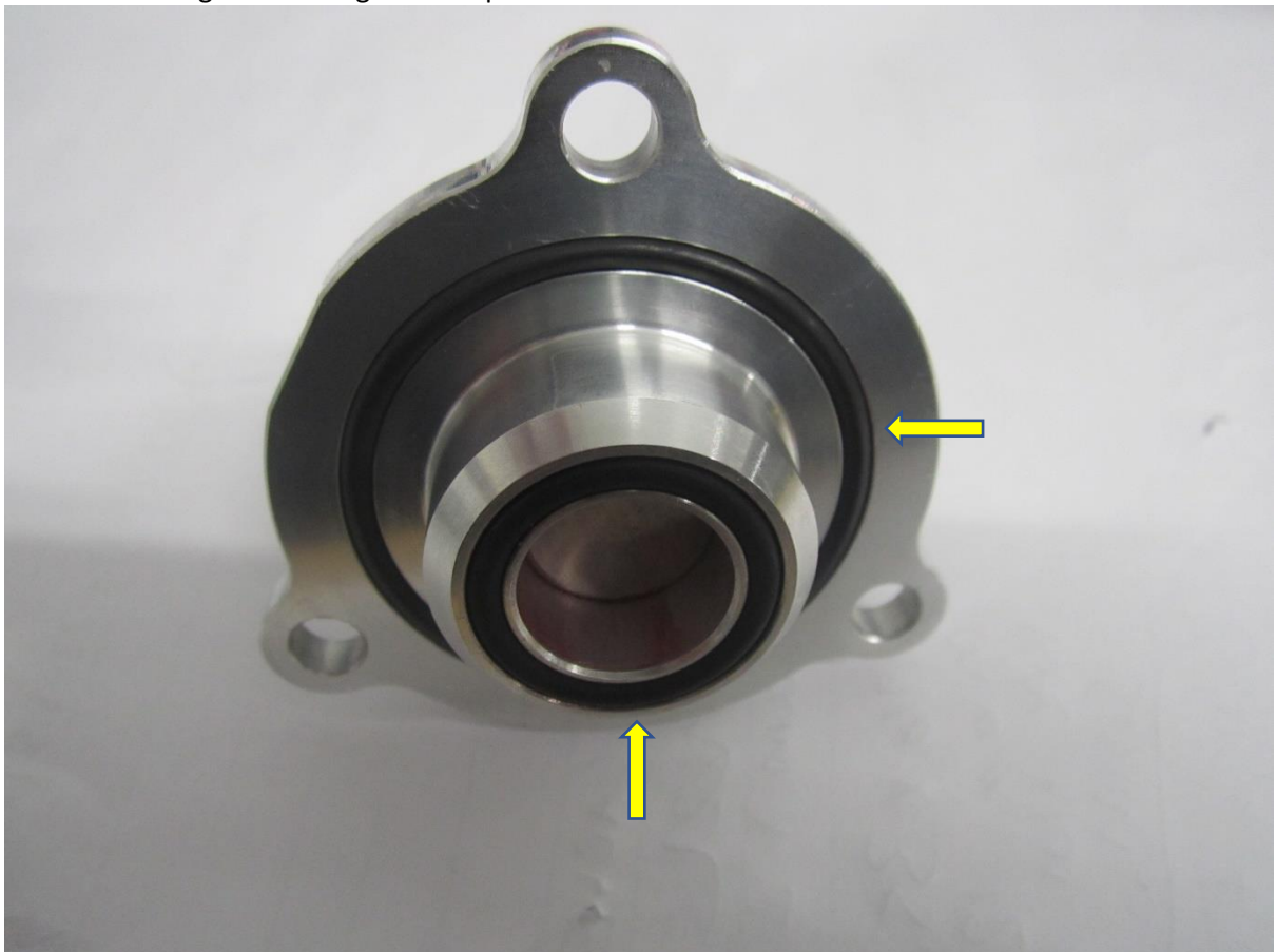
17. Fit the o-rings to the Forge Motorsport valves.
