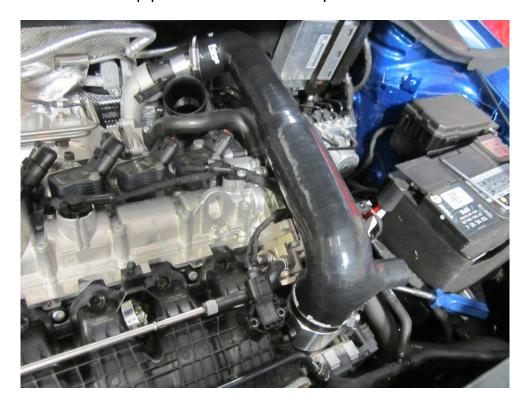
17. Now fit the new Forge Motorsport dump valve into position and tighten the hose clamp that holds it in position.
