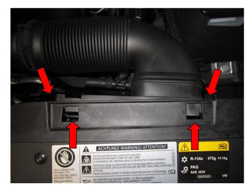
3. Remove the pipe from your airbox to the cam cover breather.
