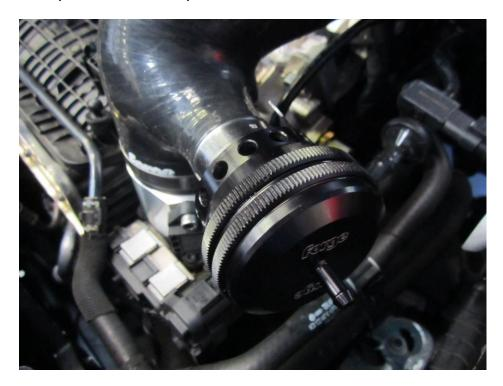
18. Now connect the vacuum pipe supplied from the top of the dump to the boost take off block you fitted in section 14. Using the tie clips provided, fasten the vacuum tube to the coolant pipe pictured and arrowed white.
