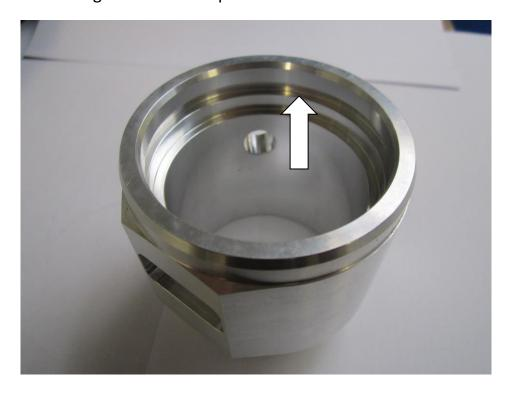
11. Now fit your coupler into position, again pushing until you hear a click. Then using a 6mm allen key, fit your MAP sensor and connect the wiring loom.
