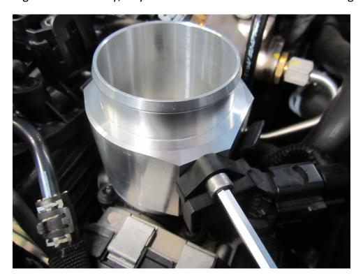
12. You must now remove the MAP sensor that's mounted in your inlet manifold. Again pry the clips apart while pulling on the sensor.
