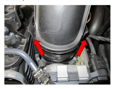
7. Unclip the opposite end of the boost pipe by again prying open the tabs arrowed red, then remove the boost pipe from its position.
