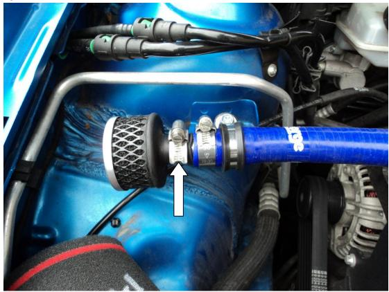
10. Fit your new intake hose and hose clamp to the turbo outlet pipe.
