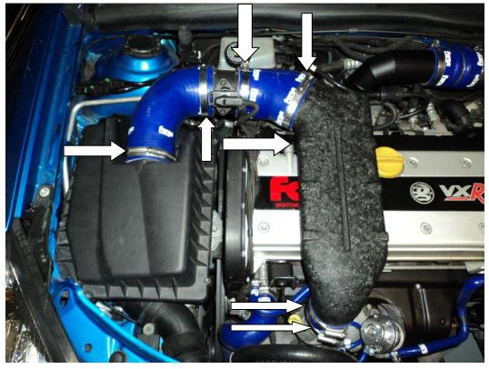
2. Unplug the wiring harness that goes to the air flow sensor by pulling on the tab.
