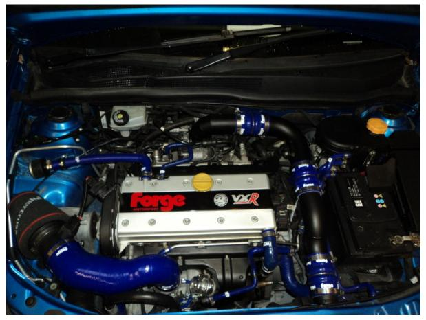
Tools Required 10mm socket with matching ratchet Hose clamp driver 1. Using a hose clamp driver, undo the hose clamps indicated in the picture below.
