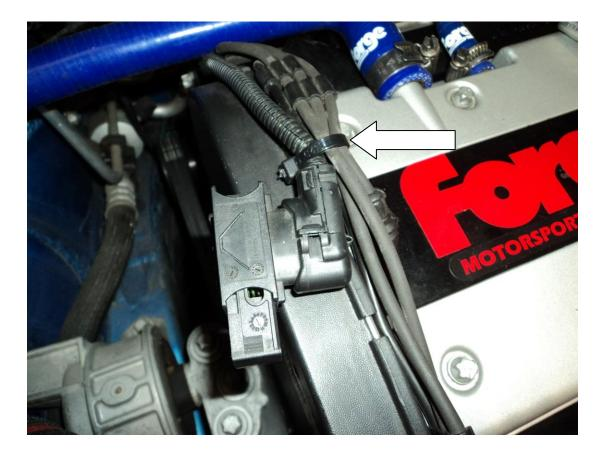
14. Attach the provided wiring harness to the air flow sensor on one end and the plug on the other.
