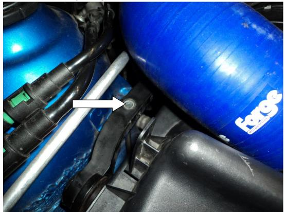
5. You can now remove the silicon pipes along with the air box.
