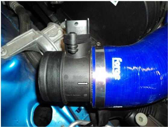
12. Fit the new Pipercross intake to the other end of the air flow sensor and tighten the hose clamp.
