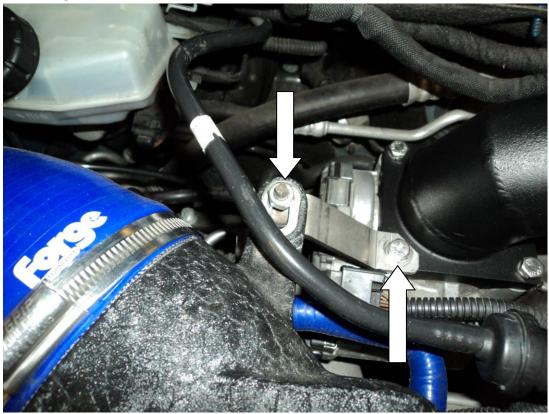
4. Remove the bolt holding the original air box to the vehicle situated at the rear of the intake.
