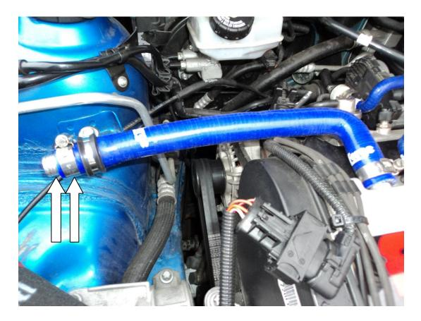
9. Now fit the oil breather filter onto the 19mm hose joiner along with a hose clamp and tighten.
