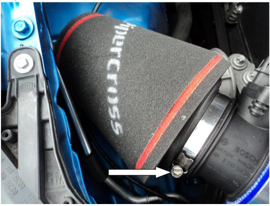
13. Place the air flow sensor plug along the top of the cam cover as seen in the picture below and using the cable tie, tie up wire to the others.
