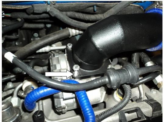
7. Fit the single ended cotton reel from where the bolt was removed in step 4.
