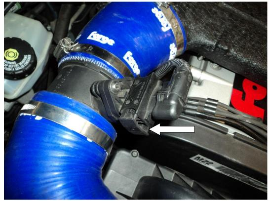
3. Undo the two 10mm bolts holding the bracket to the charge pipe. (This only applies if you have a forge intercooler).
