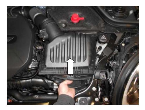
7. Using a T20 Torx driver undo the 2x screws and carefully remove the MAF sensor. Handle with care.
