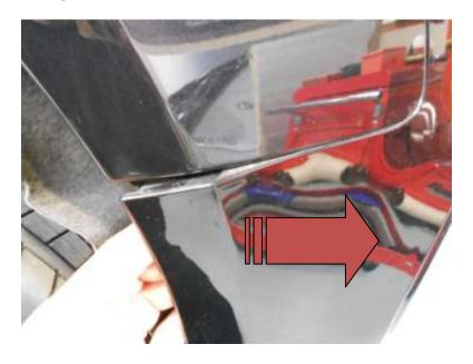
14. Using a flatblade screwdriver unclip x3 clips and remove crash bar cover.
