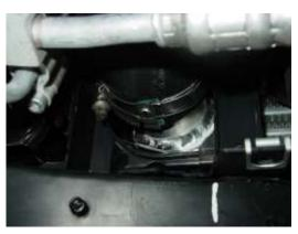
It should now be possible to slacken the hose clamps around the intercooler hoses and remove them.
