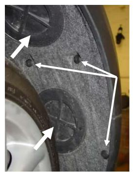
The next fasteners to be removed are those that secure the wheel arch liner at the front. With the vehicle suitably supported, and the front wheels removed it will be easier to gain access to these. Also remove the two round access covers by rotating and withdrawing.
