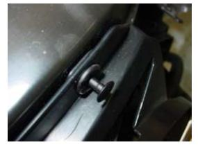
Firstly the vehicle will need to be secure and raised to allow the removal of the front wheels. The hood or bonnet of the vehicle should be opened. The grill needs to be removed. This is secured at the top edge by four plastic fasteners (push pins). The center pin of the fastener is prized out with the blade of a flat screw driver. This allows the fastener to be with withdrawn from its locating hole.
