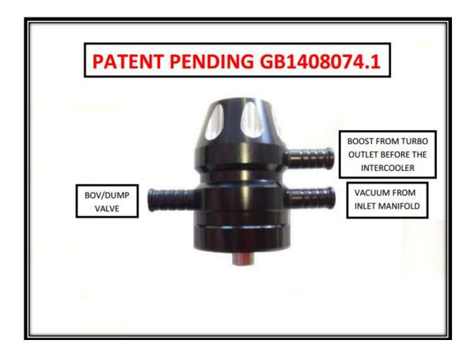
To install your IPCV, simply cut through the vacuum hose from the inlet manifold to the dump valve, connect the vacuum hose from the dump valve onto the side with the single port. Then, connect the vacuum hose from the inlet manifold to the lower port on the side with two ports. The remaining port needs to be connected to the turbo outlet, in most cases the vacuum hose connecting the actuator would be the easiest.
