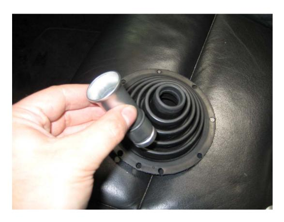
...and push the new Forge adaptor into the gaitor from underneath, exposing as many threads as possible.
