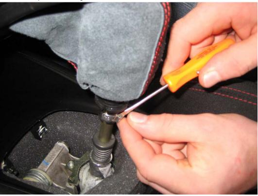
10. Pull the gaitor and gearknob up sharply and remove the whole assembly from the gearstick exposing the top of the shaft.
