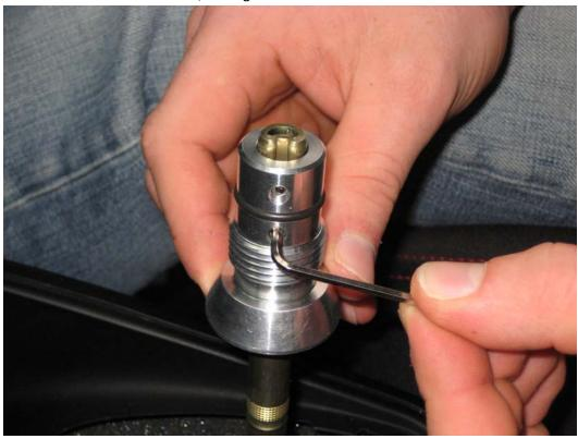
14. Pull the gaitor over the Forge adaptor until all of the threads are showing – this is a very tight fit. Refit the gaitor to the centre console.
