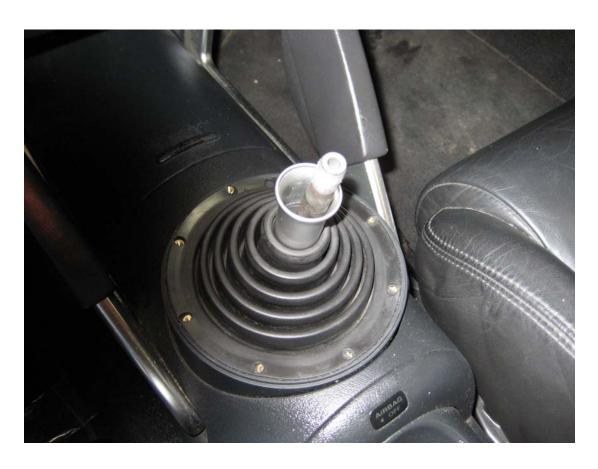
....and remove the rubber gaitor and aluminium spacer (if applicable) from the gear stick.
