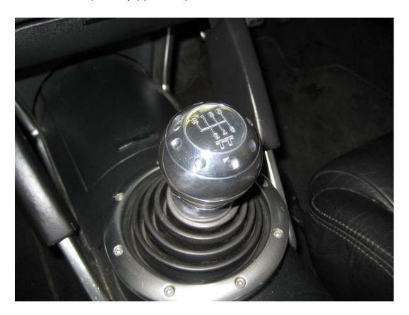
8. For cars with a SLOTTED gear knob (late Audi/Seat/VW), unclip the gaitor by pulling up at the rear and releasing from the locating lugs at the front, then pull it up as high as you can.
