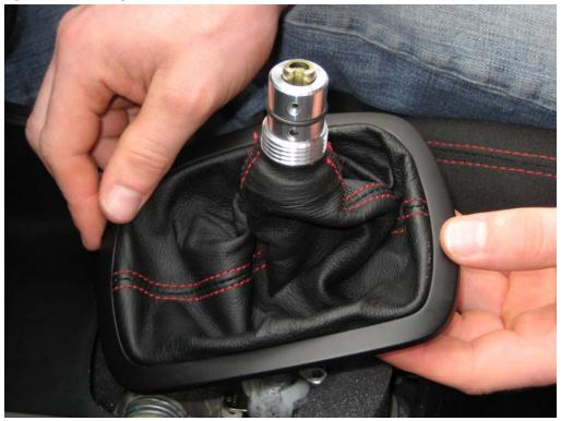
15. Screw the Forge big knob onto the adaptor and push the insert into the top of the gearknob when you have the orientation correct. Installation is complete!
