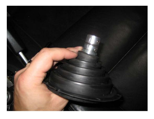
4. Replace over the shifter rod and push down until the distance between the top of the shifter rod and the top of the Forge adaptor is approx. 28mm (NB: depending on how many threads you managed to push though the gaitor, this dimension may be slightly lower or higher, however this is a good starting point)
