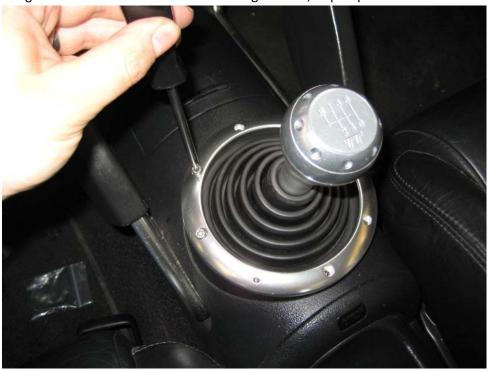
...then lift the ring away to expose the rubber underneath
