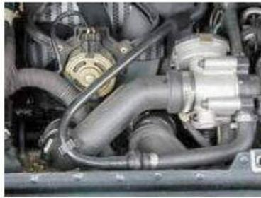
Loosen the clamps securing the intercooler pipe
