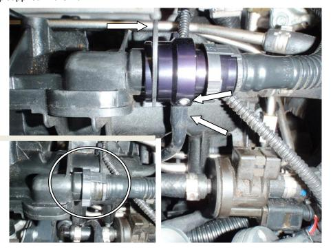
4. Using the bracket Supplied install the solenoid/bracket as shown below. You will need to plug the supplied wiring harness into the OEM Diverter valve wiring harness to do this you will need to reroute the wiring alongside the cam belt cover.
