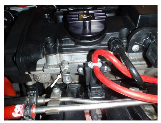
5. Remove the Plastic boost pipe by removing the hose clamps the 10mm nut and the T30 torx that secures the pipe to the engine block this can be tricky due to limited space.
