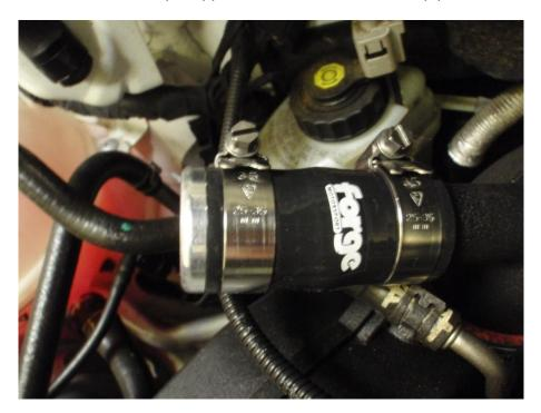
11. Forge motorsport highley recommend venting to atmosphere as this valve has a bigger bore for releasing the boost pressure. However you can install this valve recirculating if you wish. Screw in the small tube supplied in the kit and reattach the stock hose.
