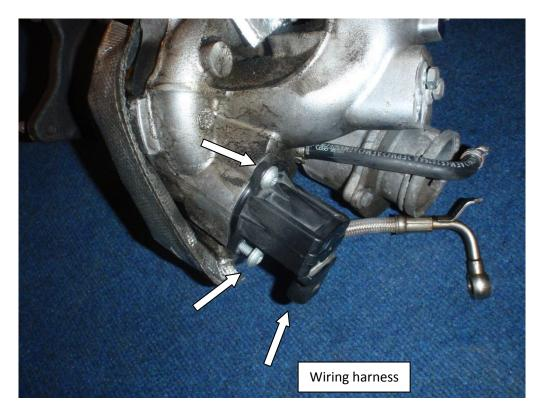
2. Fit the blanking plate to the turbo using the original dump valve torx bolts.
