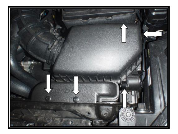
3. Undo the two bolts holding the filter box and remove. At this step the forge motorsport filter can be fitted however, if you wish to remove the rest of the Hyundai filter in the lower bumper or install the forge motorsport cold air ducting follow steps 5 to 11 and 13 to 14 to remove the bumper.
