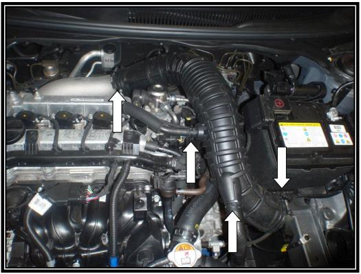
2. Push out the plastic clips and unclip the filter cover. Remove the filter cover, filter and cold air feed.
