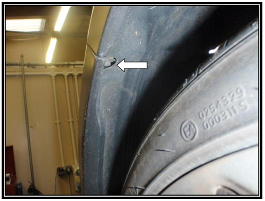
6. Using a phillips screw driver undo and remove the plastic clips on the bottom edges of the bumper.
