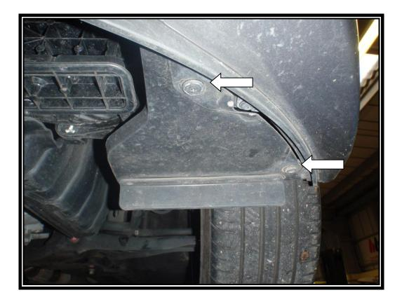
7. Pull the arch liner down and disconnect the lights.
