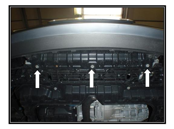
9. Undo the four bolts and unscrew the plastic clips.
