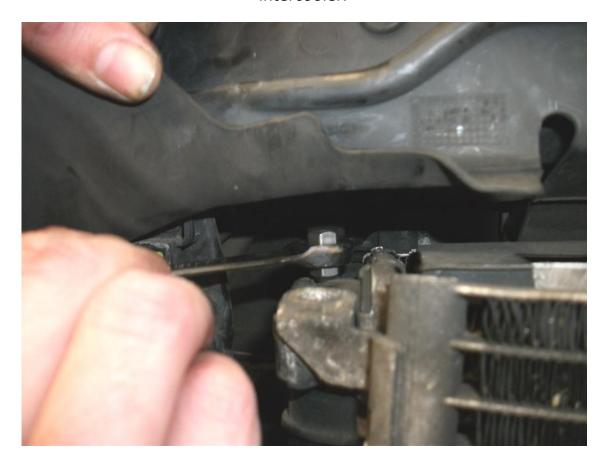
11/ Slide the air conditioning radiator up off of its brackets and move enough so that you can pull the old intercooler out.
