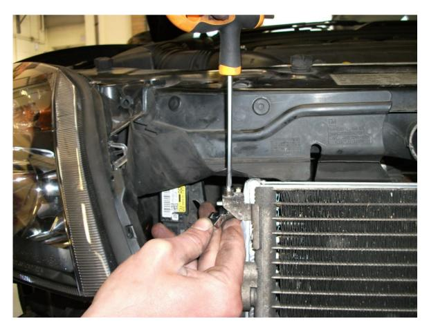
14/ Refit the Air conditioning radiator, crash bar and bumper check that all of the hose clamps are tight and test drive the vehicle.
