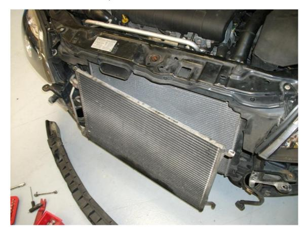
12/ Place the forge intercooler back into its place and use the supplied 5mm Allen head bolts.
