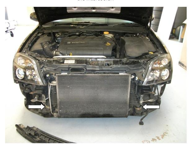
10/ Using the 10mm spanner and the T25 Torx bit remove the intercooler support bracket screws this can be tricky due to the limited space. There is one on each side of the intercooler.
