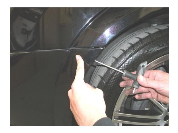
3/ Remove the three plastic body panel clips from the lower section of the bumper that connects it to the underneath of the car.
