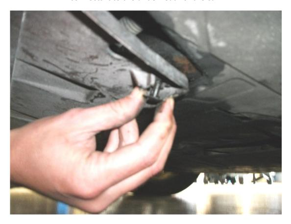
4/ Remove the three T25 Torx from each of the lower arch liners.
