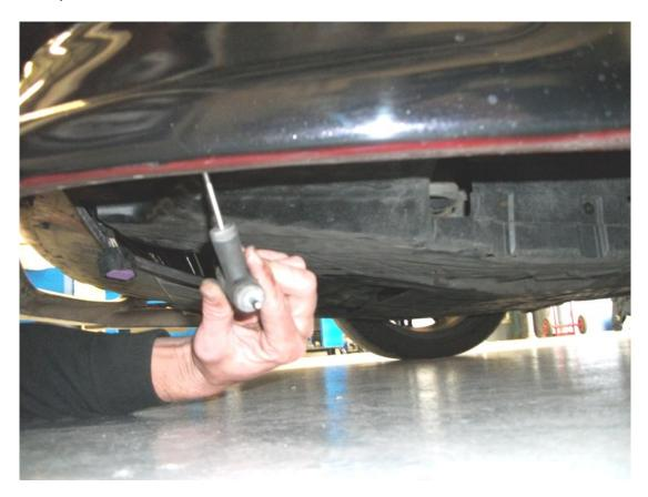
5/ Disconnect the wiring harness for the front bumper you may need to pull the bumper out slightly to access this.
