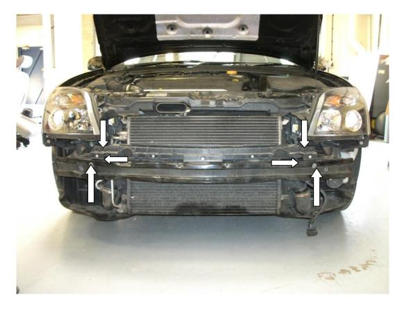
8/ Remove the air-conditioning radiator securing T25 Torx screws.
