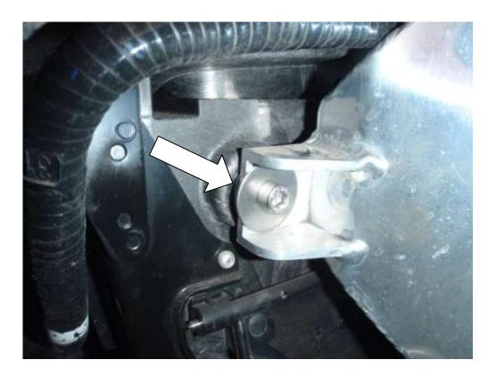
41. Remove the four rubber grommets and drain plug from the OEM radiator and install them onto the new radiator.
