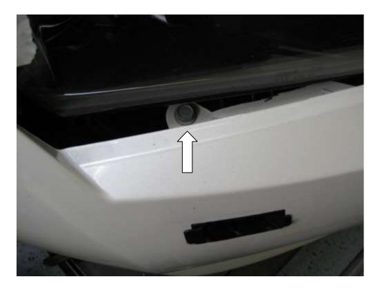
13. Push the sprung edge of the washer over to release it from the front face of the bumper, then push the washer through the hole.
