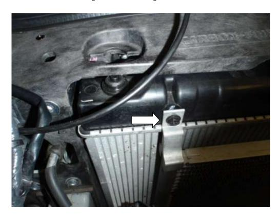
37. Lift the air conditioning up out of the bottom brackets, swing outwards out of the way of the radiator.
