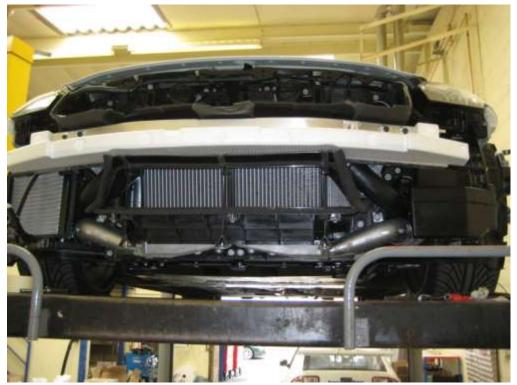
16. Remove the ducting over the oil cooler by popping out the four fixings. Remove the polystyrene bumper support by pulling it from the crash bar, then undo the six 10mm bolts on the bottom of the crash bar holding the top of the ducting for the intercooler.
