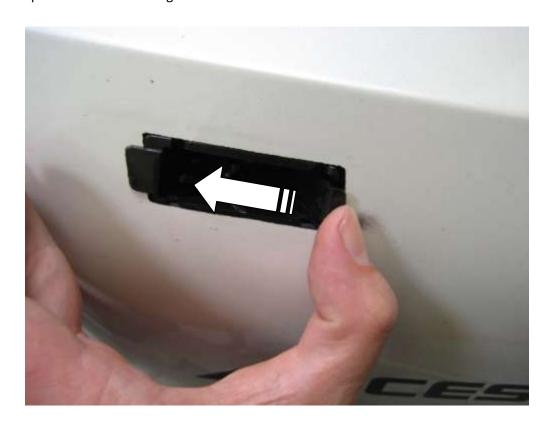
14. Ensure that the ignition is OFF, then separate the plug on the wiring harness to the crash sensors in the front bumper, which can be found on the left side of the slam panel (see picture in step 4)
