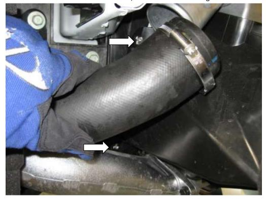
20. Remove the two bolts holding the intercooler inlet pipes to the chassis, the two bolts on the edges of the intercoolers (in the middle of the car) and one of the two top bolts of each intercooler (use a ratchet spanner), leaving one upper bolt to hold the intercoolers in.
