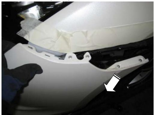
10. Clips holding the bumper on, can be removed if the bumper won't pull off the clips, by removing the two 10mm bolts as shown below.
