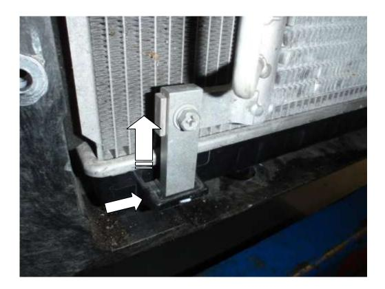
38. Tilt the radiator forward and lift out of the car.
