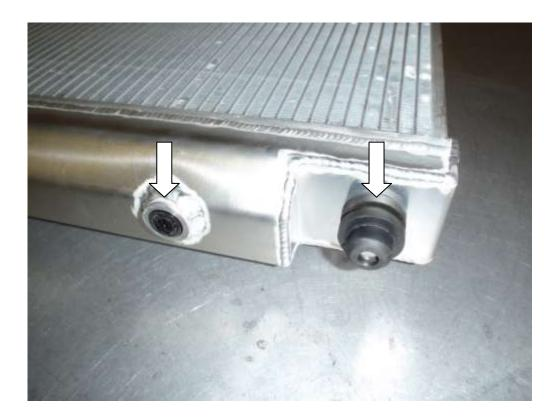
42. Install the new radiator in reverse order, following steps 38 - 28 were the oil cooler spacers need to be fitted as shown below. Continue following steps 24 - 2 to finish installation.
