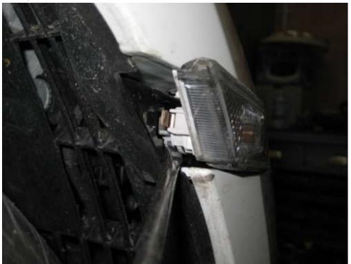
4. Remove the 4 push in clips holding the bottom edge of the arch liner to the bumper, then pull back the edge of the liner from the bumper and undo the single 10mm bolt
