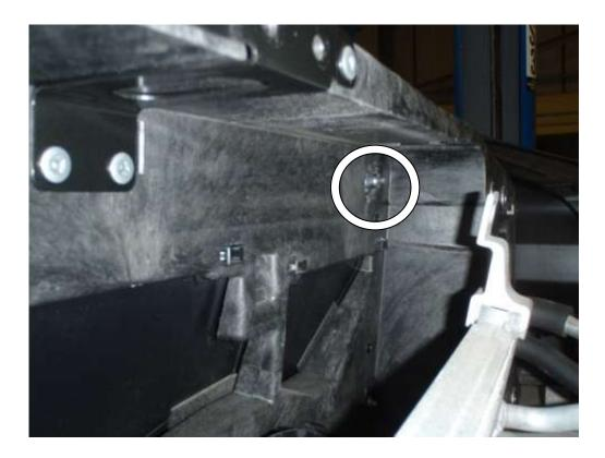
40. The smaller bolt fitted from the other side of radiator pack is on the right hand side of the header tank.
