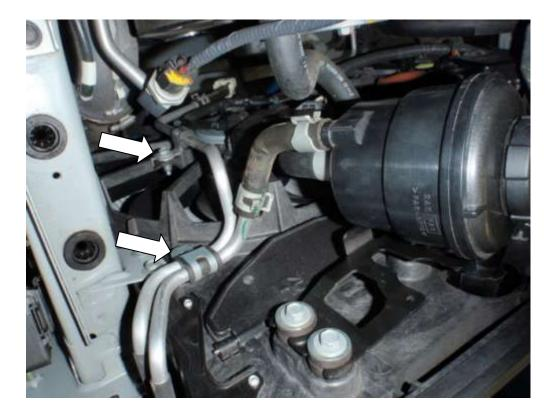
28. Undo the bolts on the power steering cooler.
