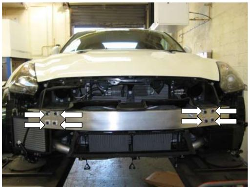
18. Remove the three supports that pass through the intercooler ducting, noting their orientation on the brackets.
