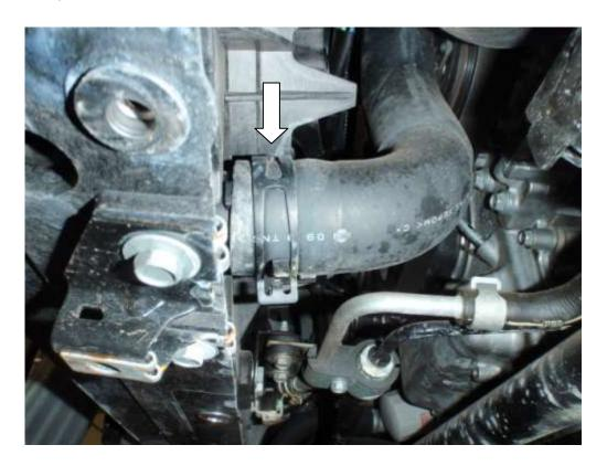
35. Unlock the radiator from the top slam panel and remove.
