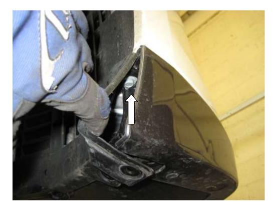
5. With the arch liner pulled out of the way, you will be able to easier access the other bolt holding the bumper to the wing. We found it easiest to use a long extension on a 3/8" drive to get onto the bolt.
