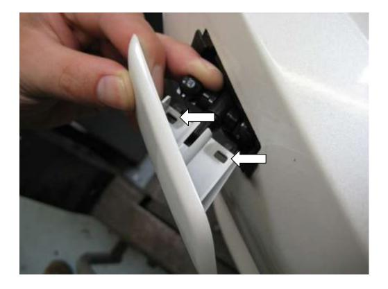
12. Pull the bumper forward and undo the 10mm bolt holding the back of the washer in place.
